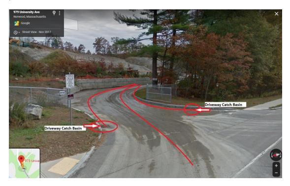
33. The Driveway Catch Basins are linked to a drainage channel that leads to the Purgatory Brook Wetlands.
