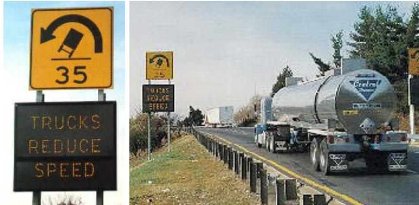
**Figure 1. A speeding truck activates the sign**
