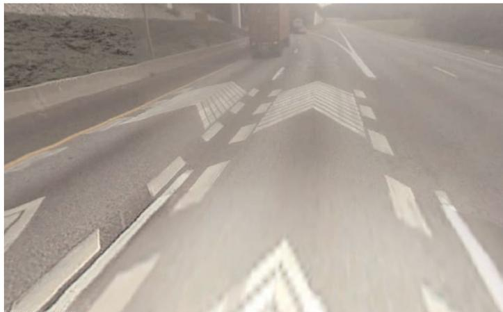
**Figure 11. Converging Chevron pavement markings in Georgia**
