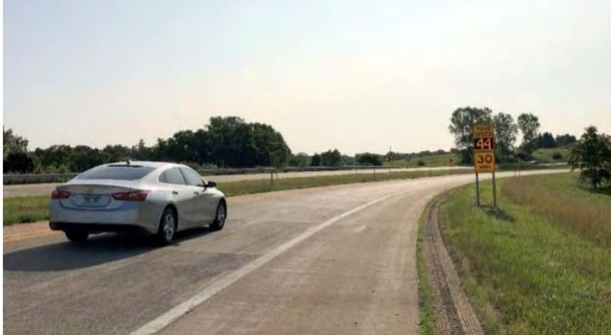
**Figure 5. Dynamic speed feedback signs with advisory speed panel**
