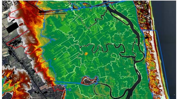
Figure 3: Visual depiction of elevations, based on LIDAR data, of salt marsh and adjacent upland areas in northern Massachusetts
