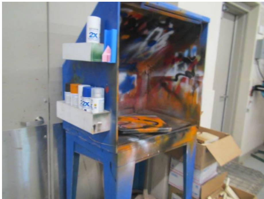
Painting spray booth in the wood shop, also note the exterior door
