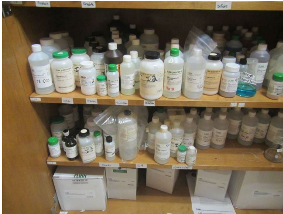
Chemicals in a science prep area cabinet, note flask on right of upper shelf with inappropriate cover
