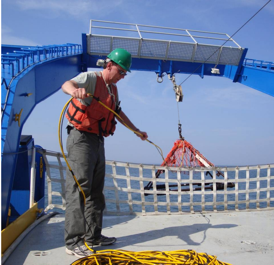
Photo: Bob Boeri (MA Coastal Zone Management) tends cable as a bottom camera is retrieved from a drop.
