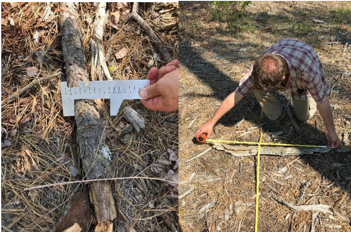
Figure 28: Example of a fuel particle inventory for A) a 100-h fuel particle tally using a go-no-go gauge and B) measuring the particle length of 1000-h fuel that intersects the transect line.
