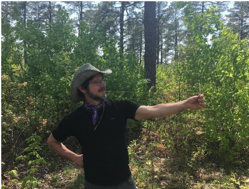
Figure 24: Using a Jim Gem Cruz All for measuring forest basal area and tree density using variable-radius plot sampling.
