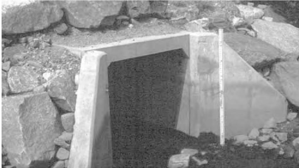
A staff gauge installed on a culvert. Photo: CZM Staff Photo
