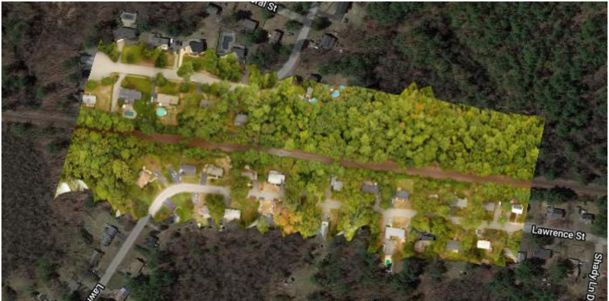
Figure 6: Multi-stereo orthophotomosaic image of rail corridor
