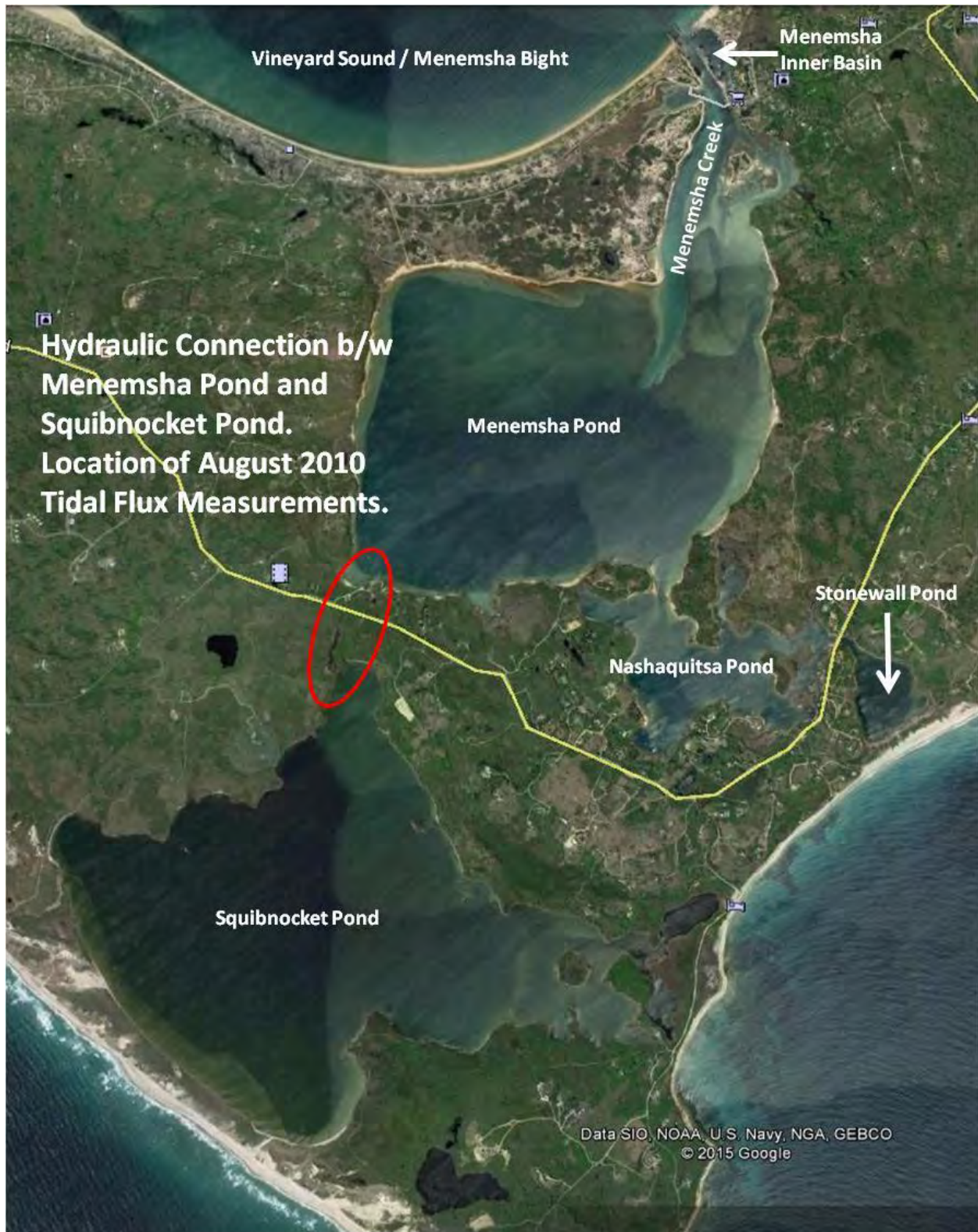
Figure IV-10 Menemsha Pond - Squibnocket Pond Embayment System. Red oval indicates the location of the herring run connecting the two basins. August 2010 tidal fluxes conducted at the culvert passing under the roadway.
