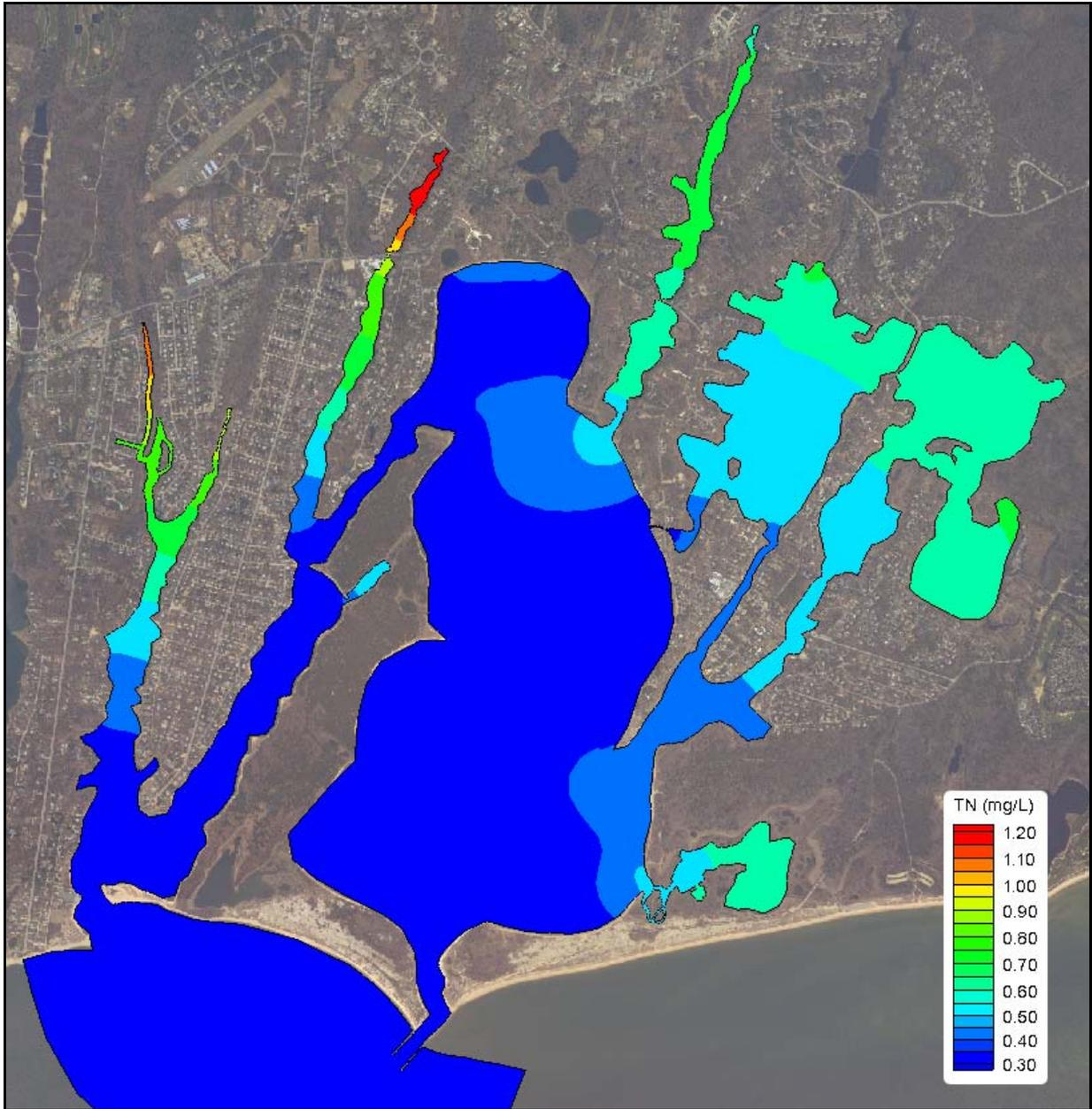
Figure VI-4. Contour plots of average total nitrogen concentrations from results of the present conditions loading scenario, for the Waquoit Bay system.
