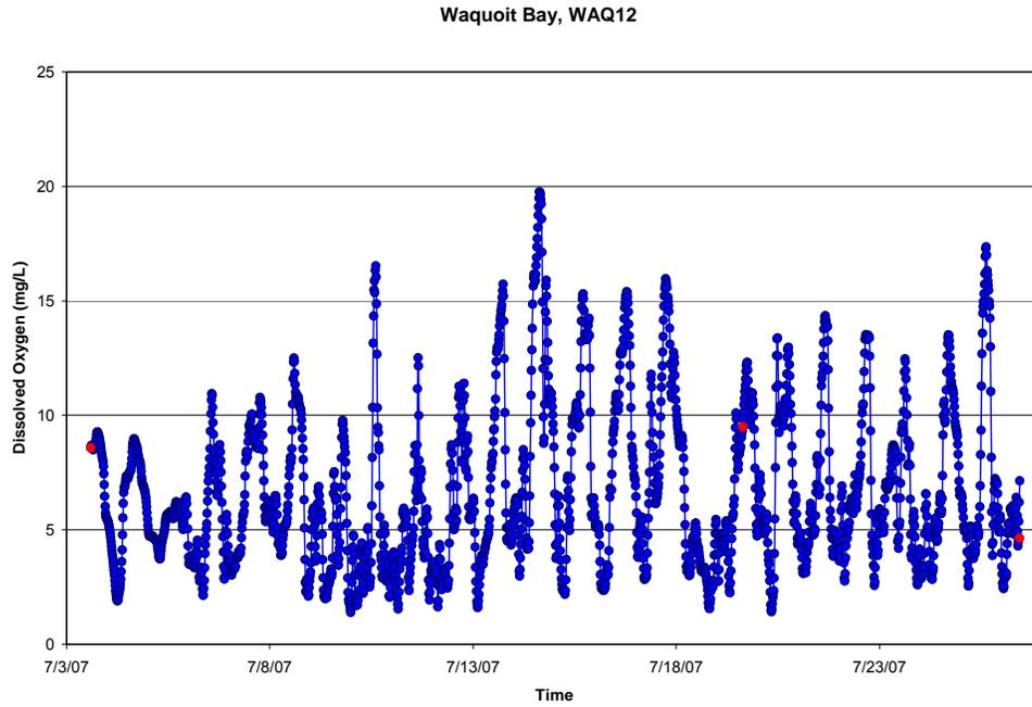
Figure VII-17. Bottom water record of dissolved oxygen within the channel of the Childs River sub-embayment (mooring WQA12), Summer 2007. Calibration samples represented as red dots.
