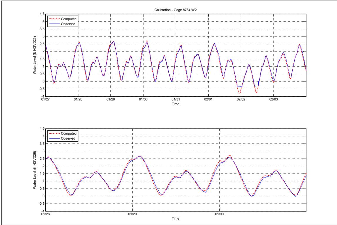
Figure V-9. Comparison of model output and measured tides for the TDR location in Eel Pond.
