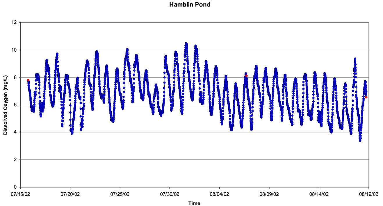
Figure VII-10. Bottom water record of dissolved oxygen (bottom panel) in Hamblin Pond, summer 2002. Calibration samples represented as red dots.
