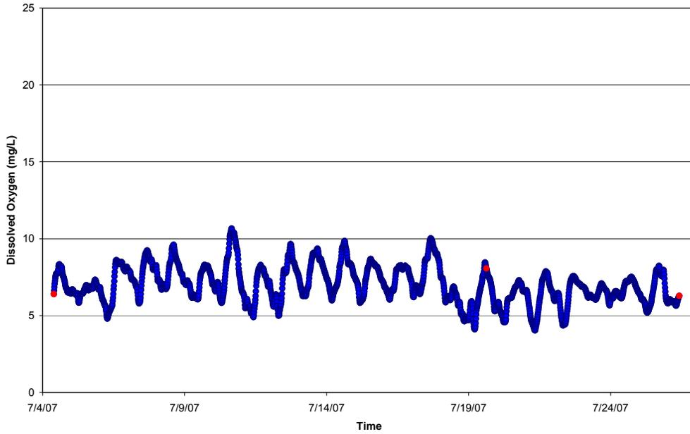
Figure VII-3. Bottom water record of dissolved oxygen at the northern mooring location in the upper tidal reach of the main basin of Waquoit Bay (WQA24), Summer 2007. Calibration samples represented as red dots.
