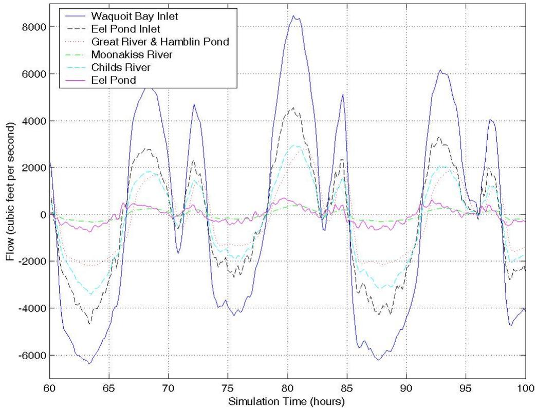
Figure V-16. Time variation of computed flow rates for six transects in the Waquoit Bay system. Model period shown corresponds to spring tide conditions, where the tide range is the largest, and resulting flow rates are correspondingly large compared to neap tide conditions. Plotted time period represents three tide cycles (12.42 h cycle). Positive flow indicated flooding tide, while negative flow indicates ebbing tide.
