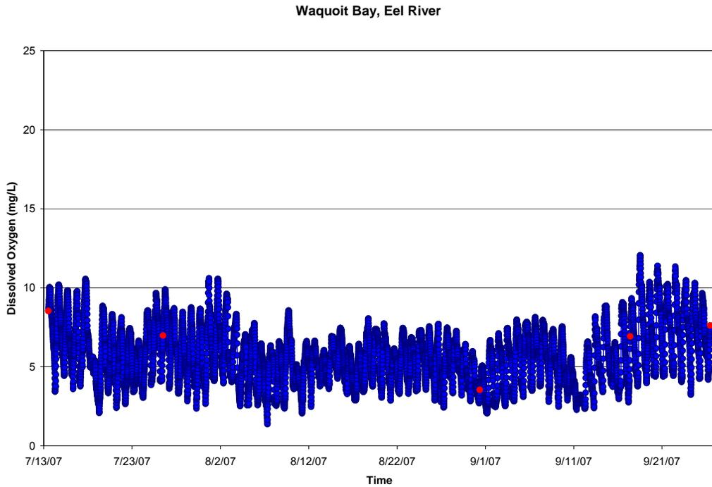
Figure VII-13. Bottom water record of dissolved oxygen within the upper reach of the west branch of the Eel Pond sub-embayment to Waquoit Bay, Summer 2007. Calibration samples represented as red dots.
