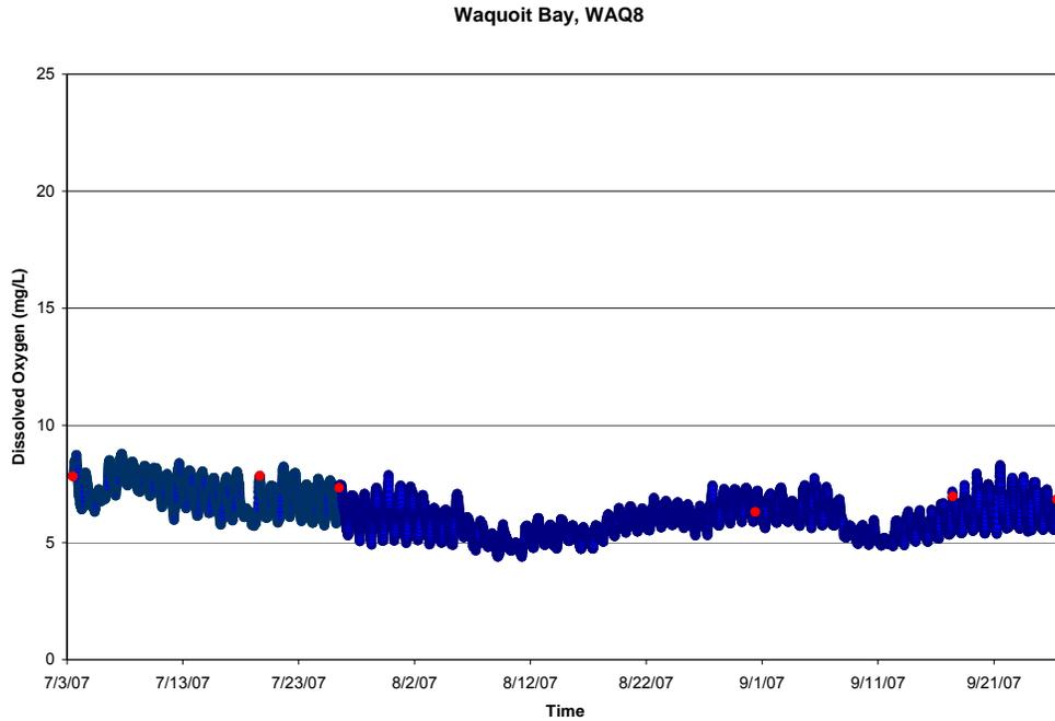
Figure VII-15. Bottom water record of dissolved oxygen within the main lower basin of Eel Pond, mooring location WAQ-8, Summer 2007. Calibration samples represented as red dots.
