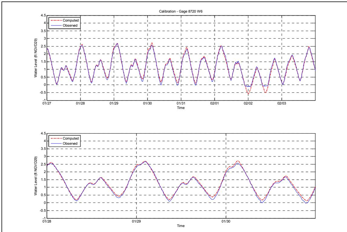
Figure V-13. Comparison of model output and measured tides for the TDR location in Hamblin Pond.
