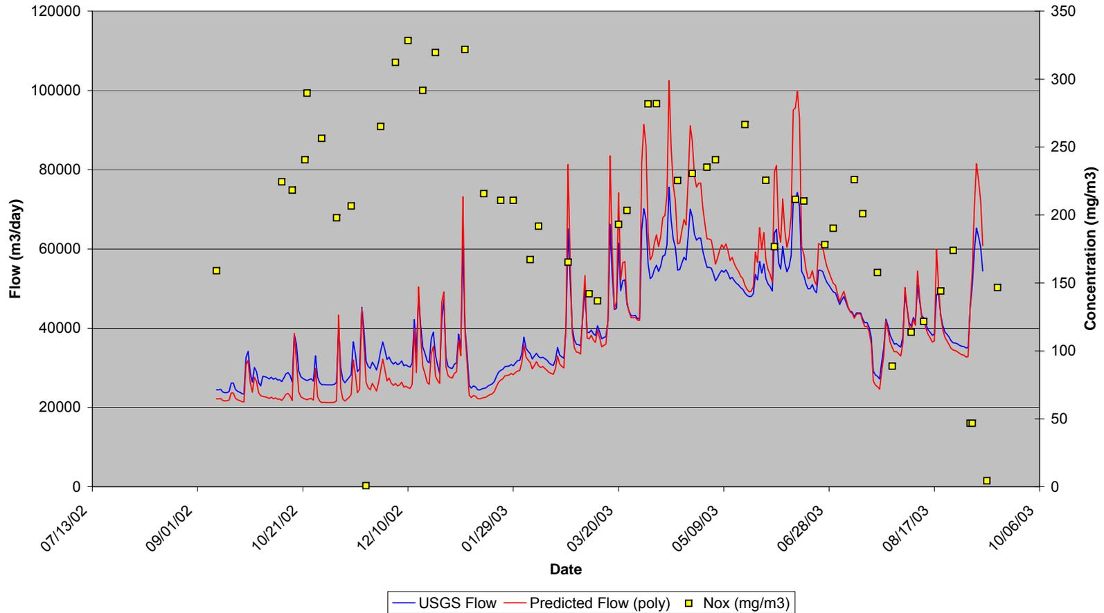
Figure IV-8. Nitrate + Nitrite (Nox) concentration and Quashnet River annual discharge developed from a stream gauge maintained in the outflow from John's Pond discharging to tidally influenced portion of Quashnet River. Nutrient samples were collected approximately weekly and analyzed for inorganic and organic nitrogen species. These data were used to determine both annual flow and total nitrogen transport for determining nitrogen attenuation (see Table IV-4).
