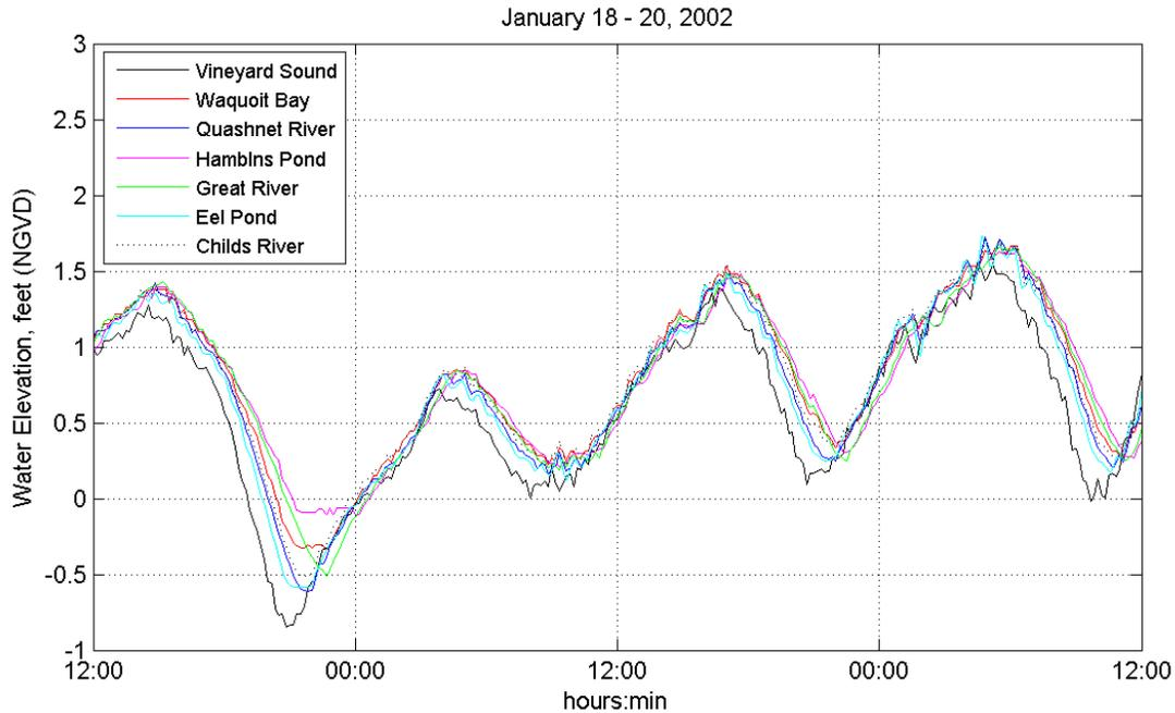
Figure V-6. Comparison of water surface elevation observations for Vineyard Sound (offshore), and six locations within the Waquoit Bay system. Damping effects are seen as a decrease in the tidal amplitude, as well as a lag in the time of high and low tides from Vineyard Sound.
