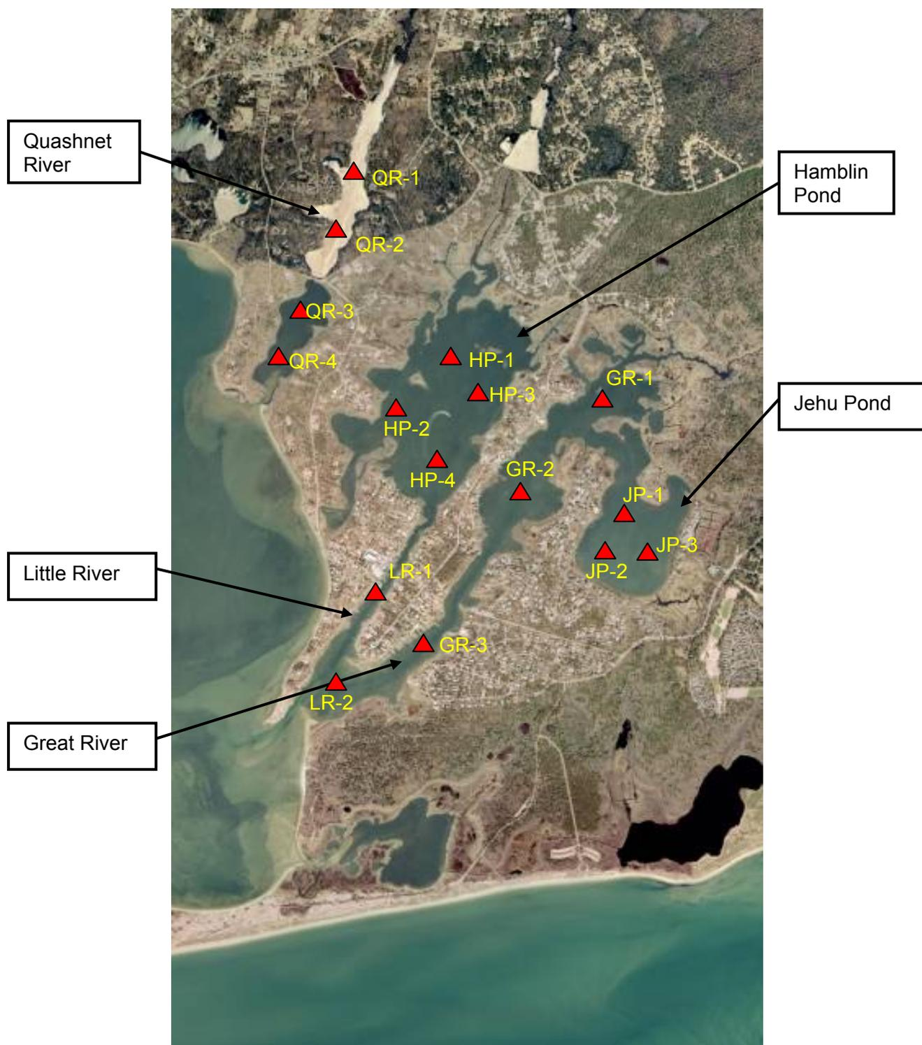
Figure IV-10. Quashnet River, Hamblin Pond/Little River and Jehu Pond/Great River sub-embayments to the Waquoit Bay System, locations (red triangles) of sediment sample collection for determination of nitrogen regeneration rates. Numbers are for reference to Table IV-8.
