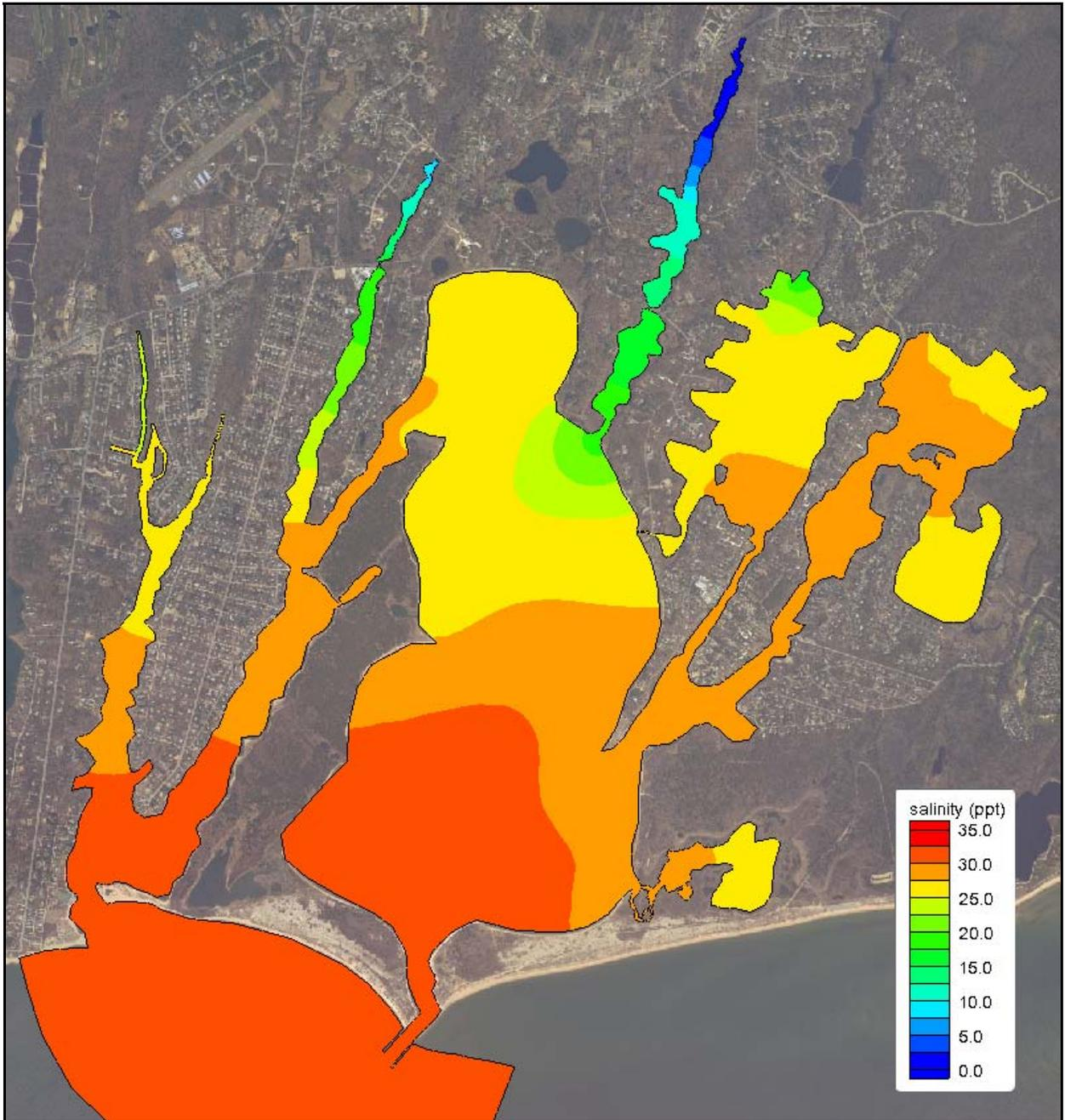
Figure VI-7. Contour plots of modeled salinity (ppt) from the model of the Waquoit Bay system.
