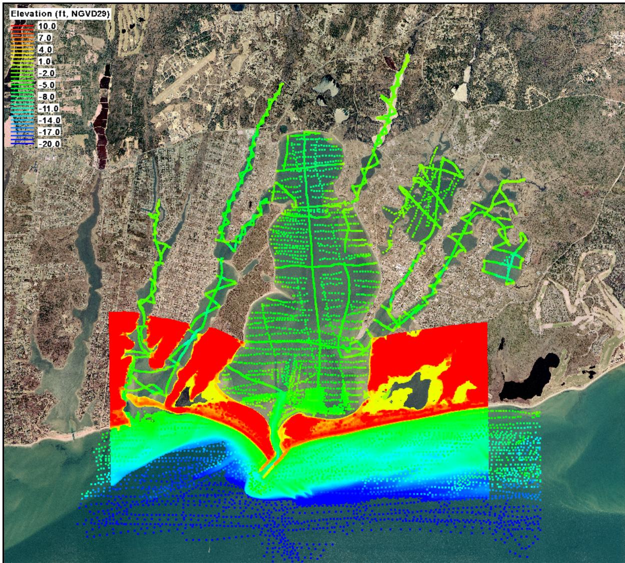
Figure V-3. Bathymetric data interpolated to the finite element mesh of hydrodynamic model, elevation is relative to NGVD29.
