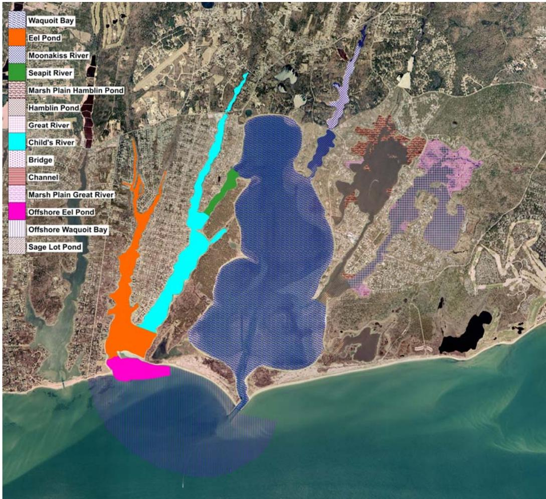
Figure V-8. Hydrodynamic model grid material properties. Color patterns designate the different model material types used to vary model calibration parameters and compute flushing rates.
