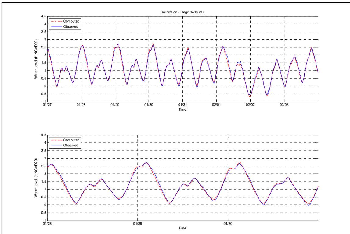
Figure V-14. Comparison of model output and measured tides for the TDR location in Great River.
