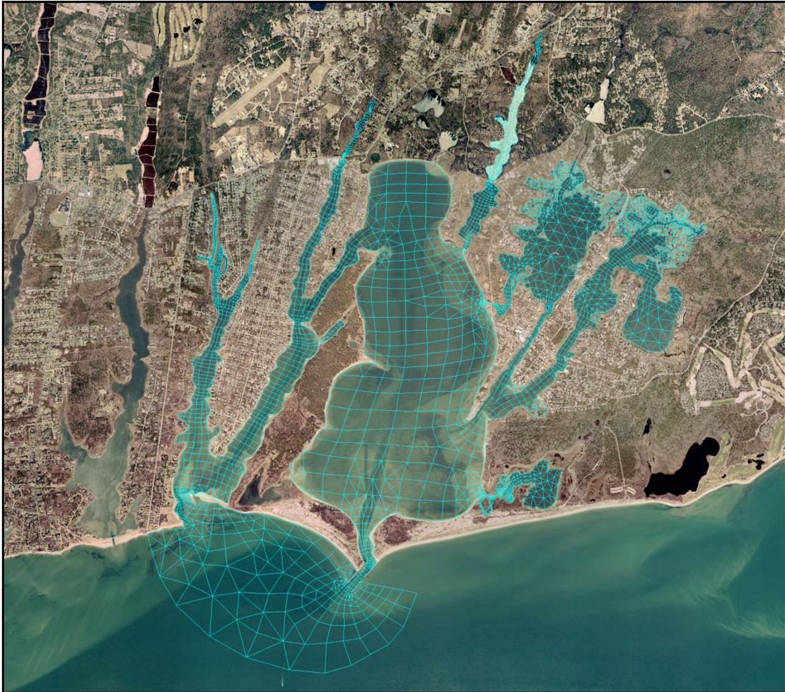
Figure V-7. Plot of hydrodynamic model grid mesh for the Waquoit Bay system.
