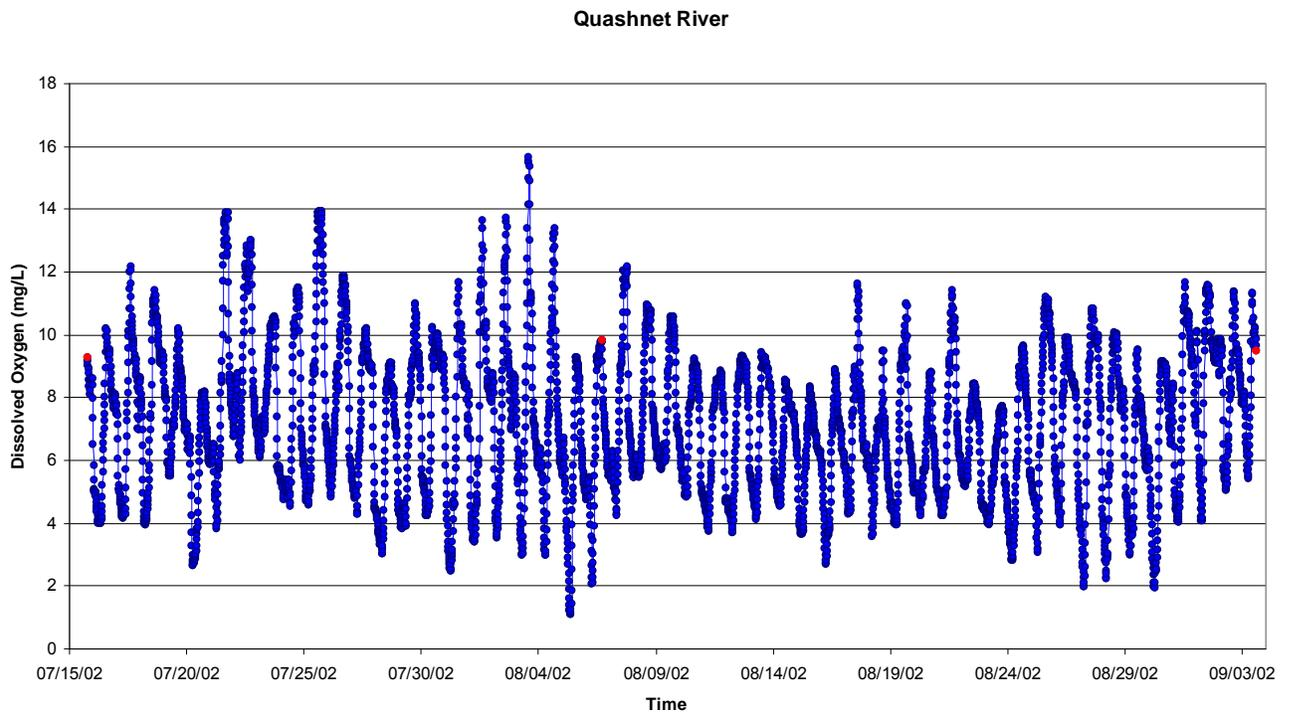
Figure VII-9. Bottom water record of dissolved oxygen (top panel) in the Quashnet River Estuary (lower basin), summer 2002. Calibration samples represented as red dots.
