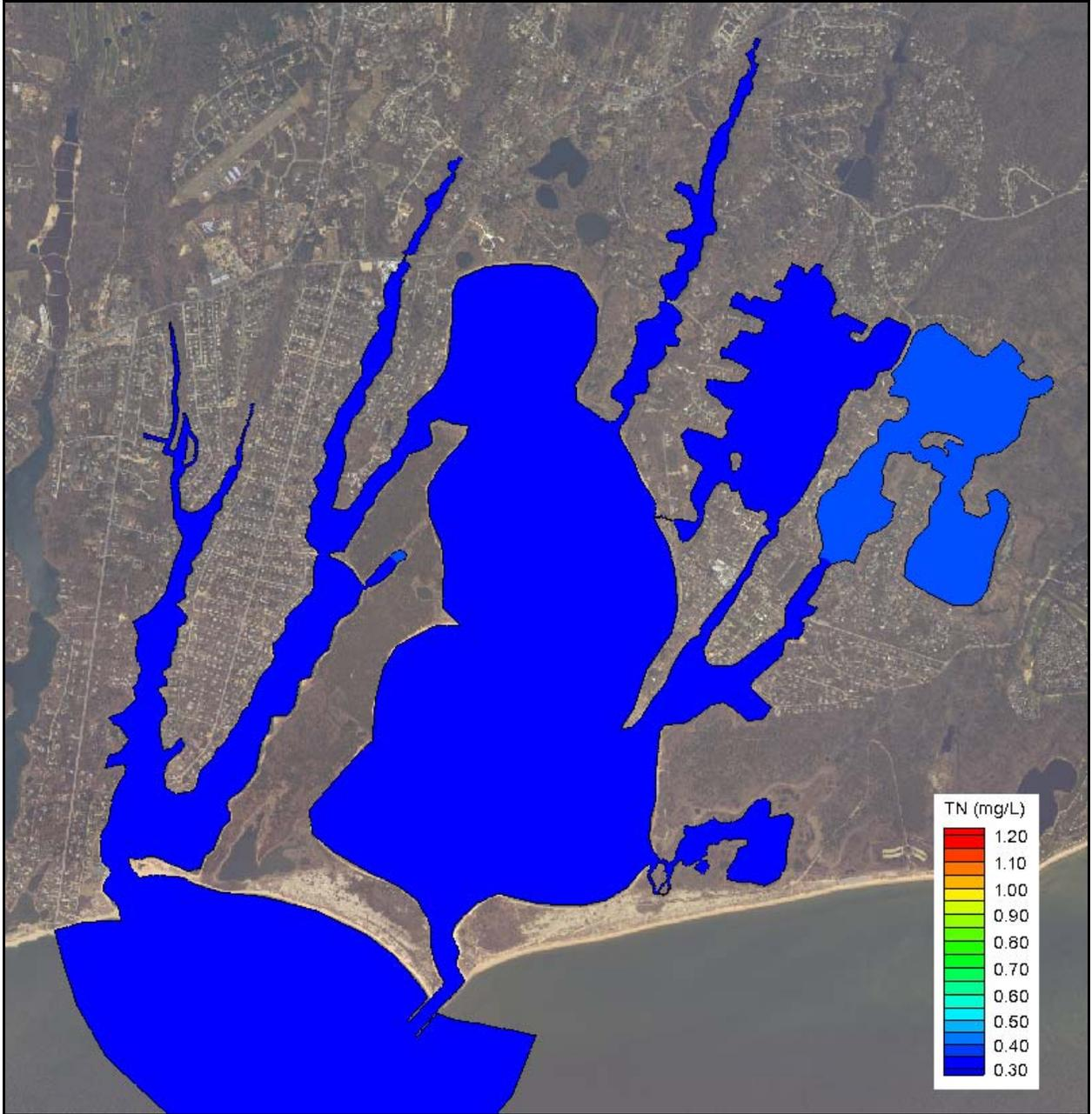
Figure VI-9. Contour plots of modeled total nitrogen concentrations (mg/L) in Waquoit Bay system, for no anthropogenic loading conditions, and bathymetry.
