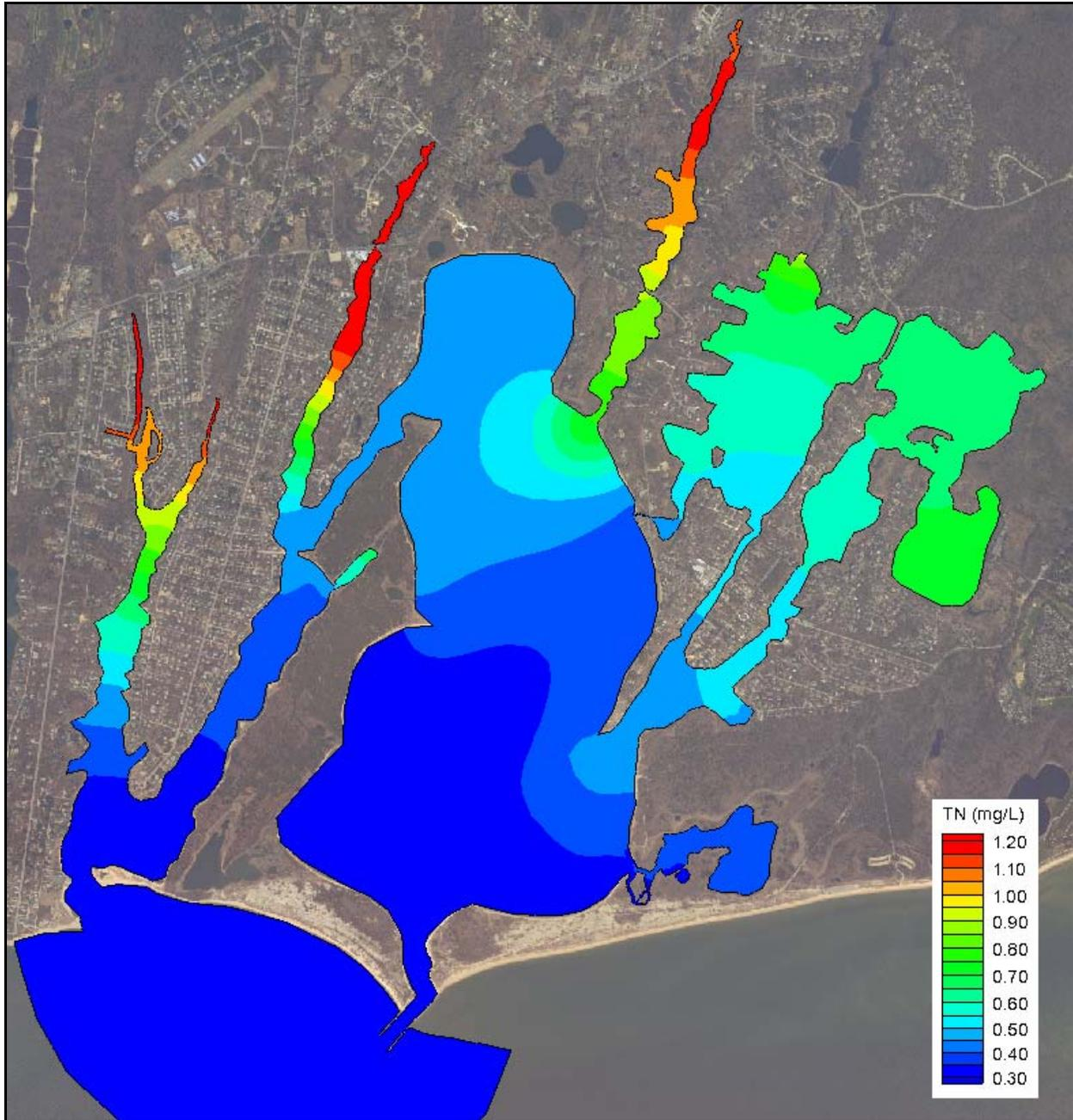
Figure VI-8. Contour plots of modeled total nitrogen concentrations (mg/L) in Waquoit Bay system, for projected build-out loading conditions, and bathymetry.
