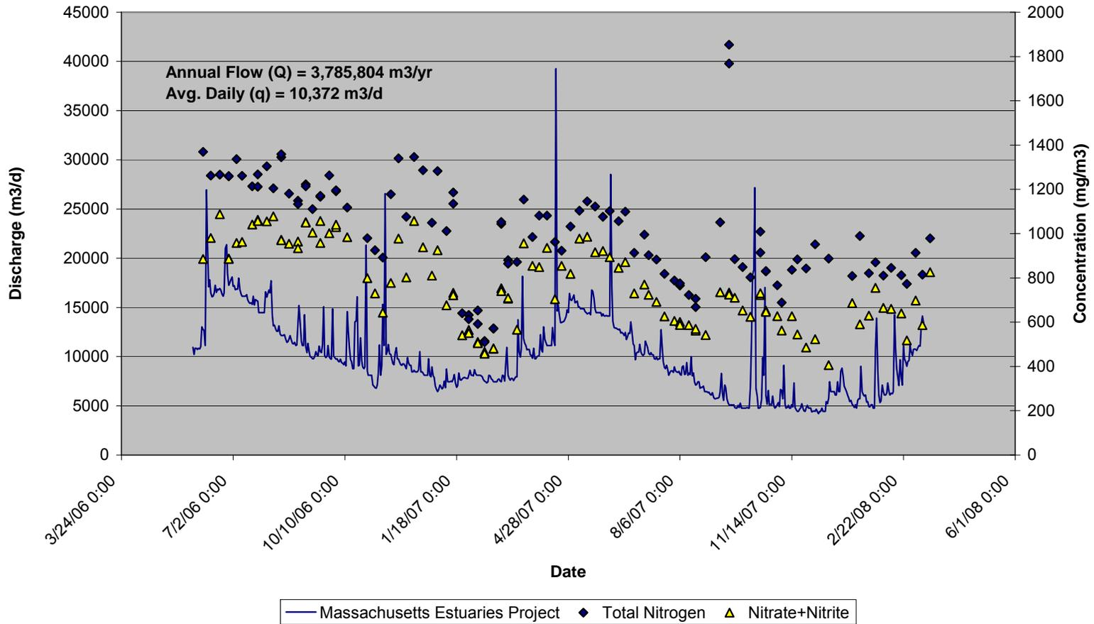
Figure IV-9. Discharge from Childs River (solid blue line), total nitrogen (blue symbols) and NO<sub>x</sub> (yellow symbols) concentrations for determination of annual volumetric discharge and nitrogen load from the sub-watershed of Childs River discharging to the head of the East Branch of the Eel Pond Sub-embayment to the Waquoit Bay Estuary (Table IV-6).
