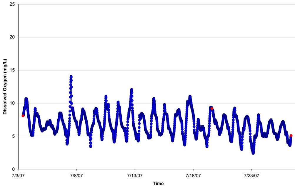
Figure VII-7. Bottom water record of dissolved oxygen within the lower region of the main basin of Waquoit Bay (WQA27), Summer 2007. Calibration samples represented as red dots.
