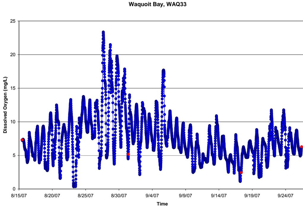
Figure VII-5. Bottom water record of dissolved oxygen within the mid region of the main basin of Waquoit Bay (WQA33), Summer 2007. Calibration samples represented as red dots.
