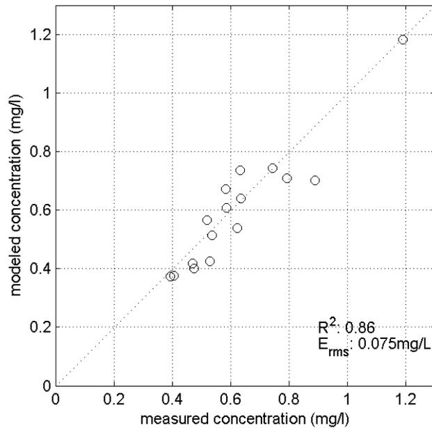
Figure VI-3. Model calibration target values are plotted against measured concentrations, together with the unity line.
