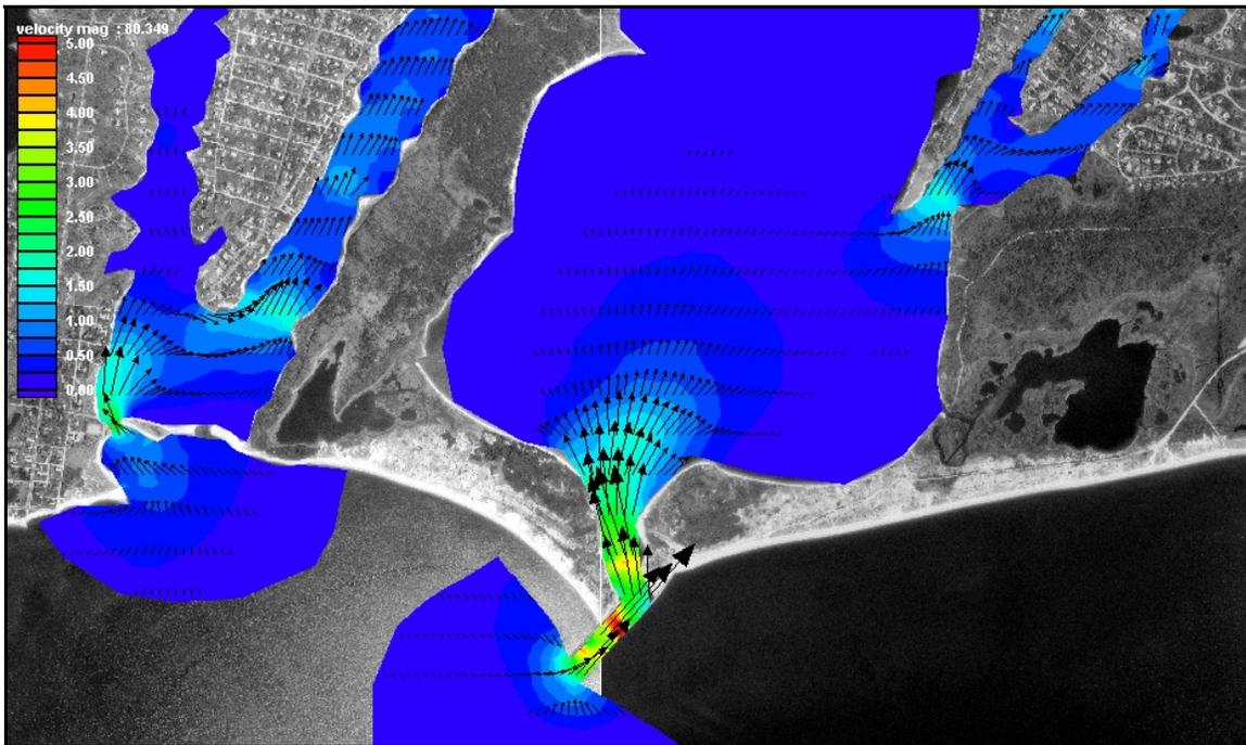
Figure V-15. Example of hydrodynamic model output for a single time step where maximum flood velocities occur for this tide cycle. Color contours indicate velocity magnitude, and vectors indicate the direction of flow.
