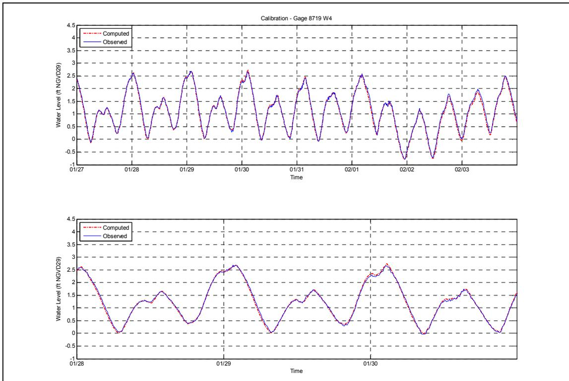
Figure V-10. Comparison of model output and measured tides for the TDR location in Childs River.
