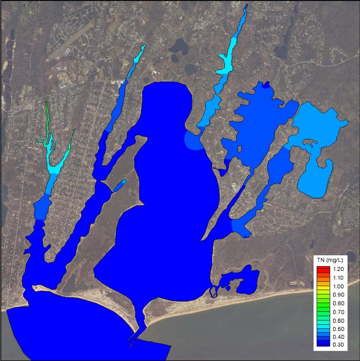
Figure VIII-1. Contour plot of tidally averaged modeled total nitrogen concentrations (mg/L) in the Waquoit Bay estuarine system, for threshold.
