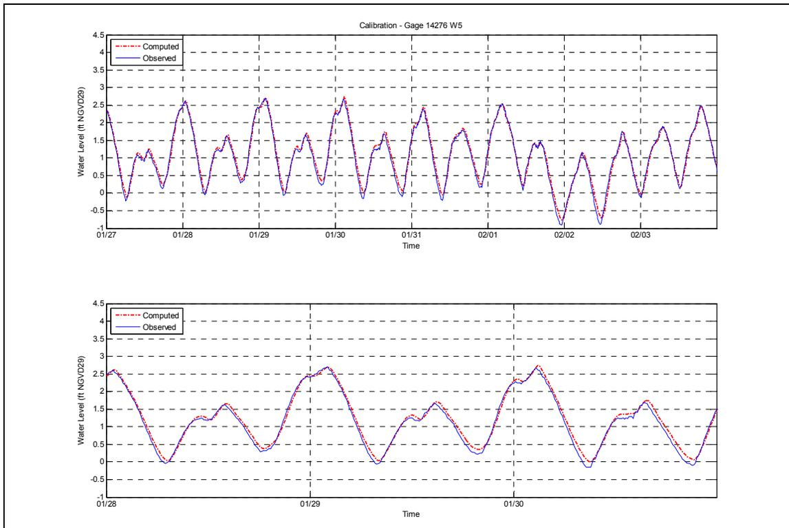
Figure V-12. Comparison of model output and measured tides for the TDR location in Quashnet River.
