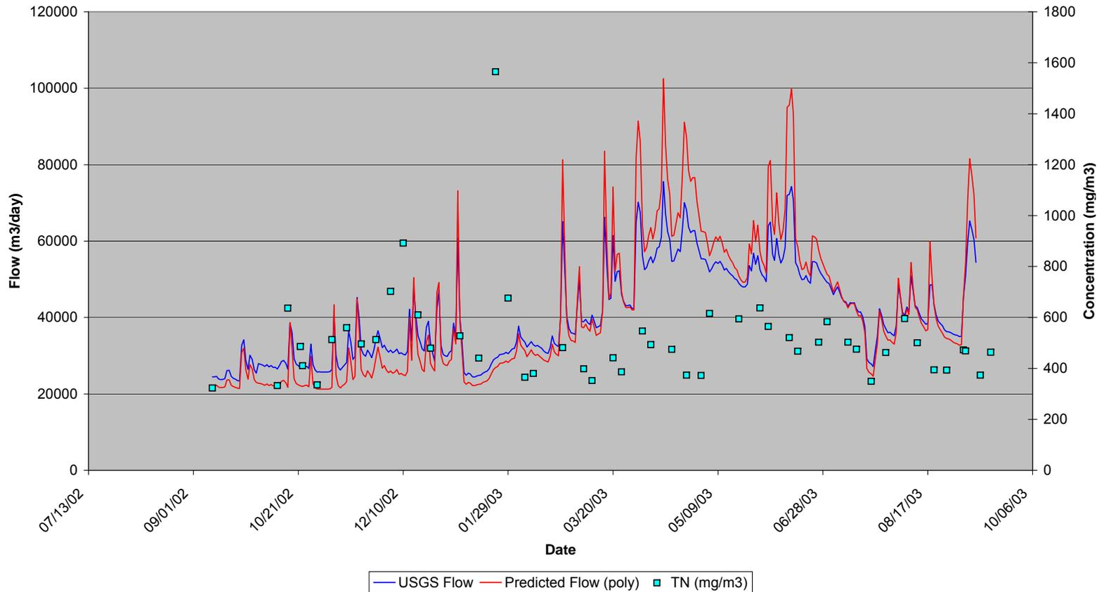
Figure IV-7. Quashnet River annual discharge developed from a stream gauge maintained above the tidal reach of the lower Mashpee River estuarine waters. Nutrient samples were collected weekly and analyzed for inorganic and organic nitrogen species. These data were used to determine both annual flow and total nitrogen transport for determining nitrogen attenuation (see Table IV-4).
