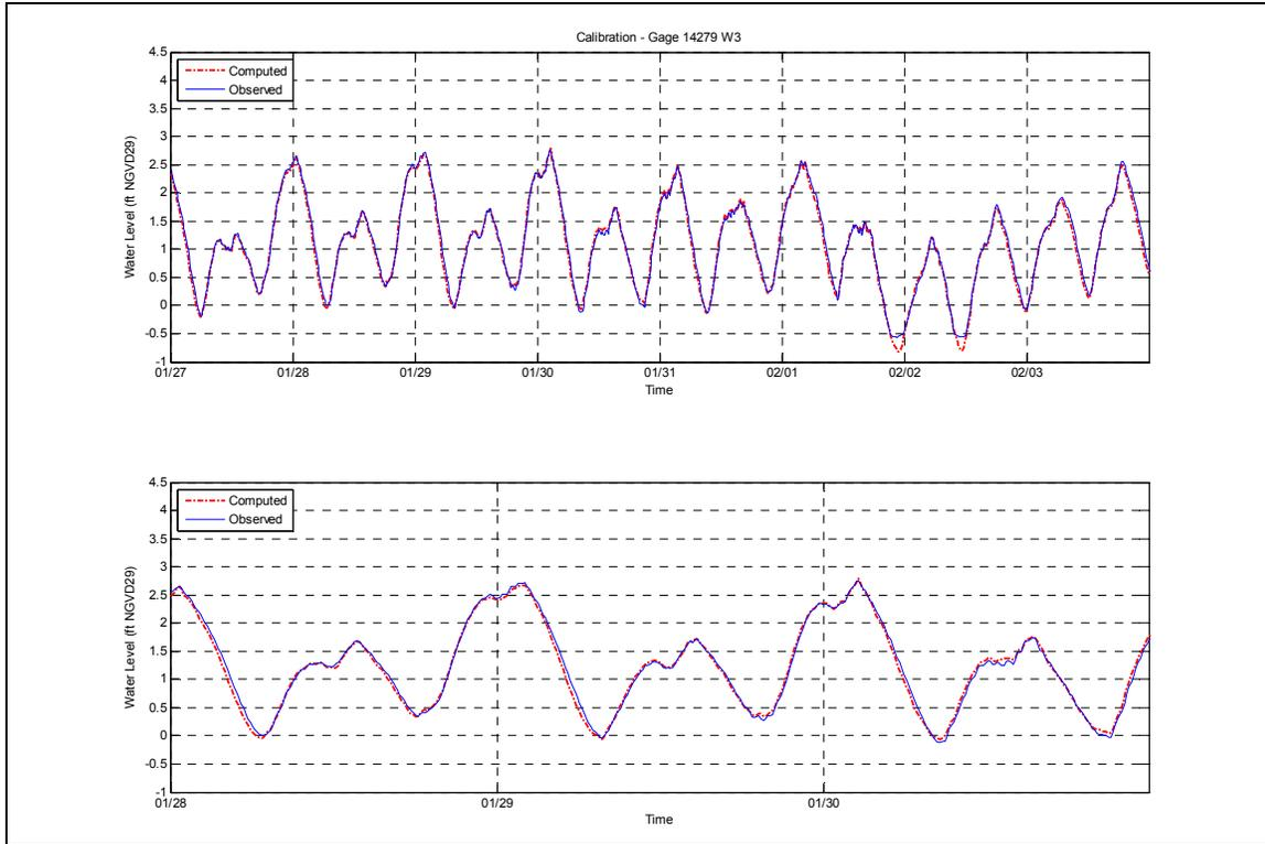
Figure V-11. Comparison of model output and measured tides for the TDR location in Waquoit Bay.
