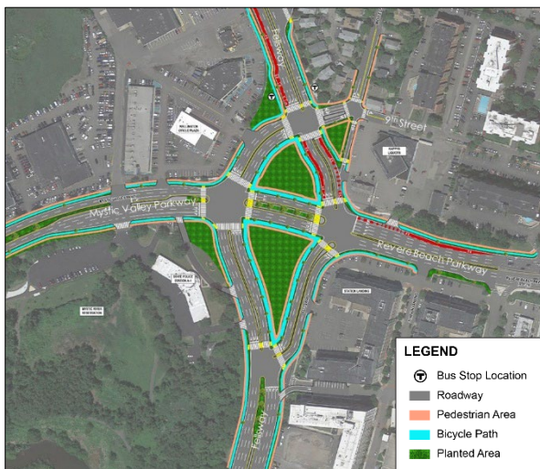
Figure 3: Long-Term At-Grade Transit Enhanced Dual Quadrant
