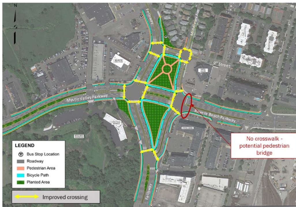
Figure 4.2-13: Long-Term At-Grade Square Pedestrian Connectivity
