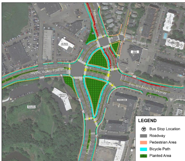
Figure 3: Long-Term At-Grade Transit Enhanced Dual Quadrant
