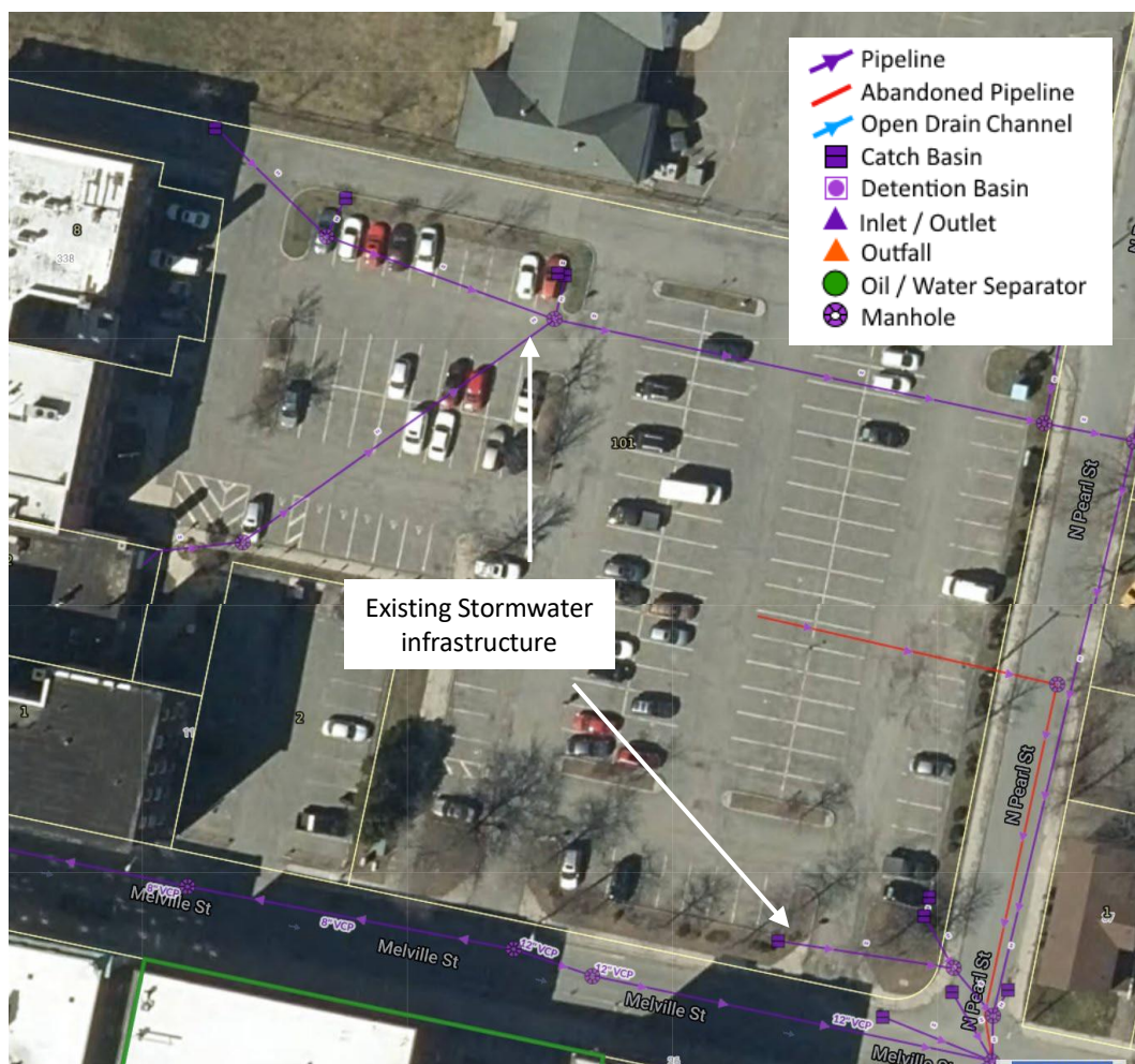
Figure C-29: Melville Street Municipal Parking lot Project Existing Stormwater Infrastructure
