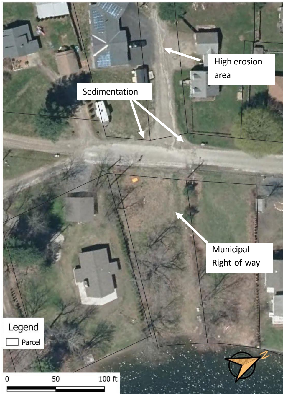
Figure C-11: Algonquin Street/Narragansett Avenue existing site conditions.
