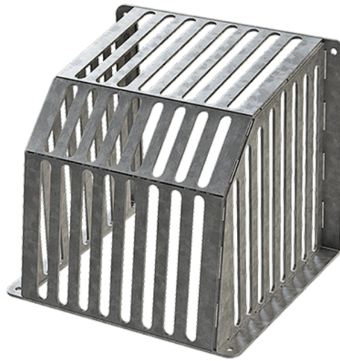
Figure 6: Trash guard which has a high surface area to retain high flow rates as trash debris accumulates. (Source: www.trashracks.com )
