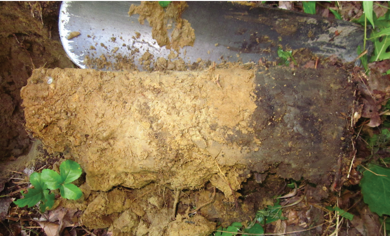
The soil profile did not exhibit indicators of saturation or anaerobic condition in the topsoil or the subsoil, therefore it did not meet the
