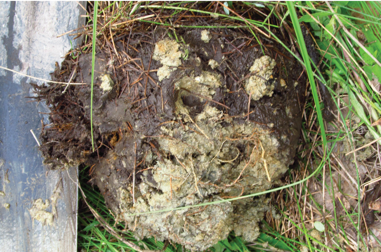
The distinct and abrupt color change in this soil profile identifies the boundary between the placed soil above and the extant (native) soil below. The shallow placed topsoil is newly forming; however, the extant subsoil is gleyed (and occurs within 12" of the surface),
