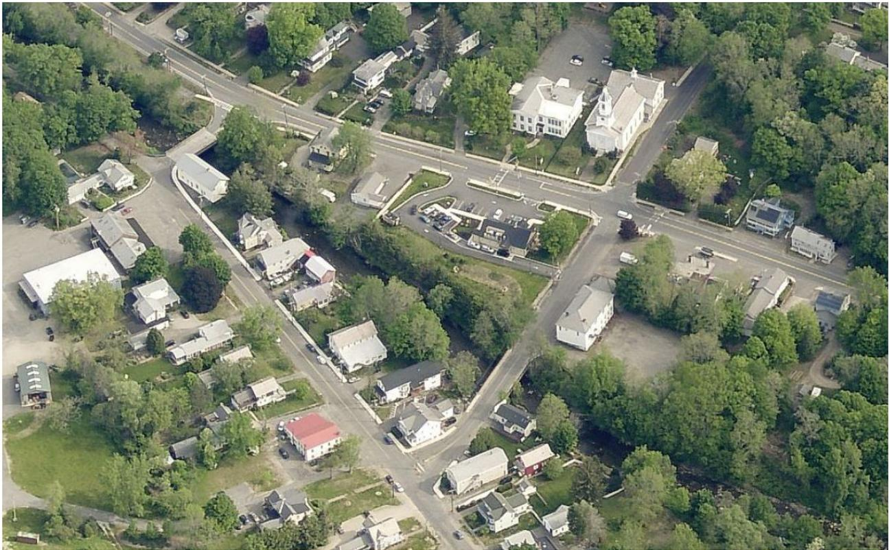
*This bird's-eye view of Haydenville shows the close relationship between the village center and the river. The Bridge Street and South Main Street bridges shown are at risk of scouring and occasional overtopping during severe storms. A current MassDOT project is redesigning the bridges.*
