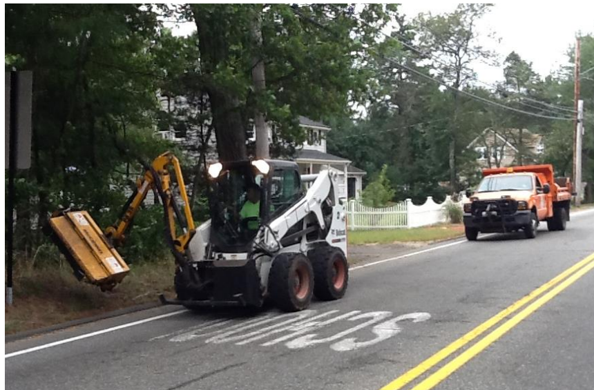
Figure 5 –Mechanical flail mower currently in use by Wilmington DPW crews
