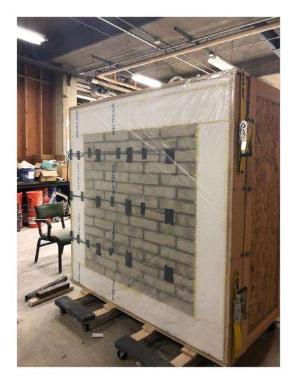
At  $\Delta$  T = 20°, DWB resistance to heat flow (R) = 4 times published value for reinforced fully grouted CMU walls.
