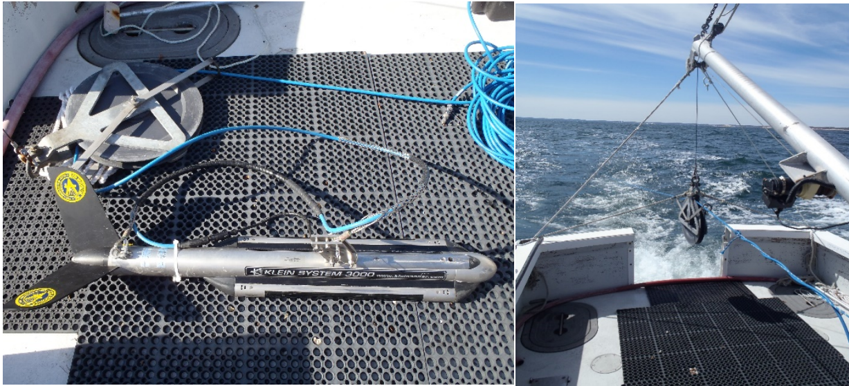
Figure 2. Klein 3000 Digital Beam side scan sonar (left). Side scan deployment setup (right).
