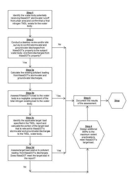
Figure 1. Flow Chart Illustrating MassDOT's Nitrogen TMDL Method
