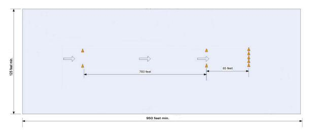
Student Evaluation: Students should be able to bring the vehicle to a complete stop in less than 100 feet at 50 mph. Proficiency shall be established when a student makes a minimum of two successful emergency braking maneuvers without striking the barrier. At the completion of the drill instructors should review what has been learned and how it will be incorporated into other drills.
