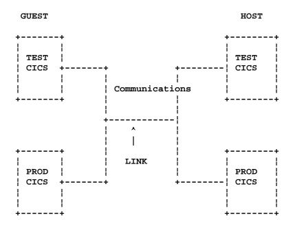
**NOTE:** Test system is connected to test system and production system is connected to production system.
