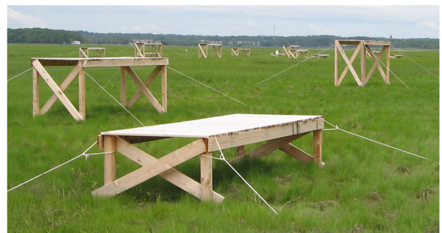
Fig. 2 Image of a single block of the experimental dock array layout consisting of docks set at height-to-width ratios ( H:W ) of 0.5:1 (low), 1:1 (intermediate), and 1.5:1 (high) above the marsh platform as well as an unshaded control plot. Four replicate blocks were installed over the low marsh ( L1 – L4 ) and high marsh ( H1 – H4 ). Treatments within each block were separated by approximately 7.5 m
