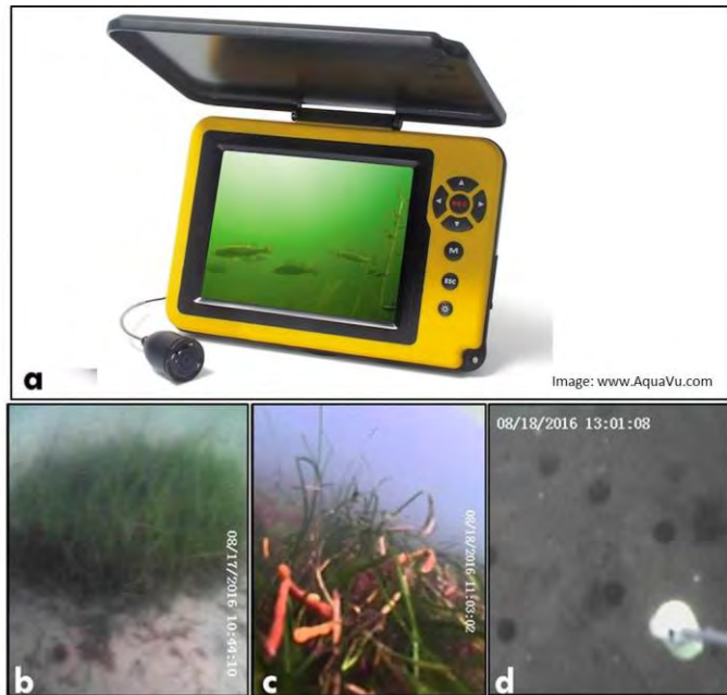
Figure 7. A) Aqua-Vu camera, B, C) imagery captured in vegetated areas, D) imagery captured in an un-vegetated area. Imagery from Salem Sound, MA.
