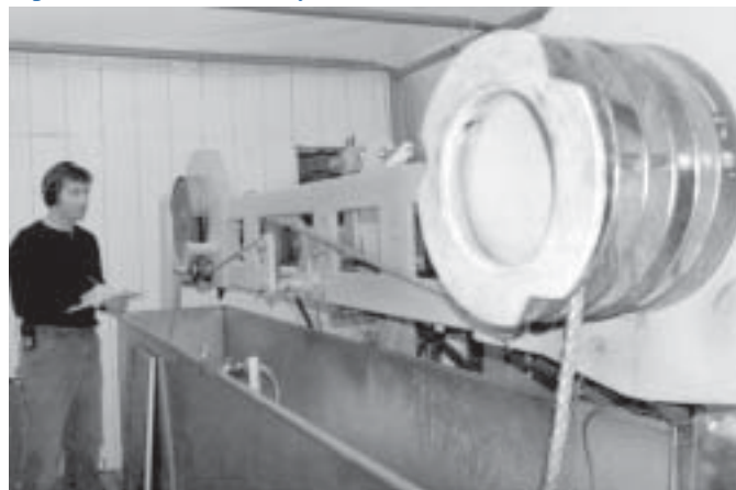
The line-testing machine that simulates years of wear within hours.
