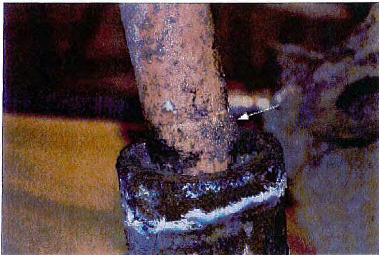
Figure 27: The dimpled region was the source of the leak, not the transition fitting, arrow.
