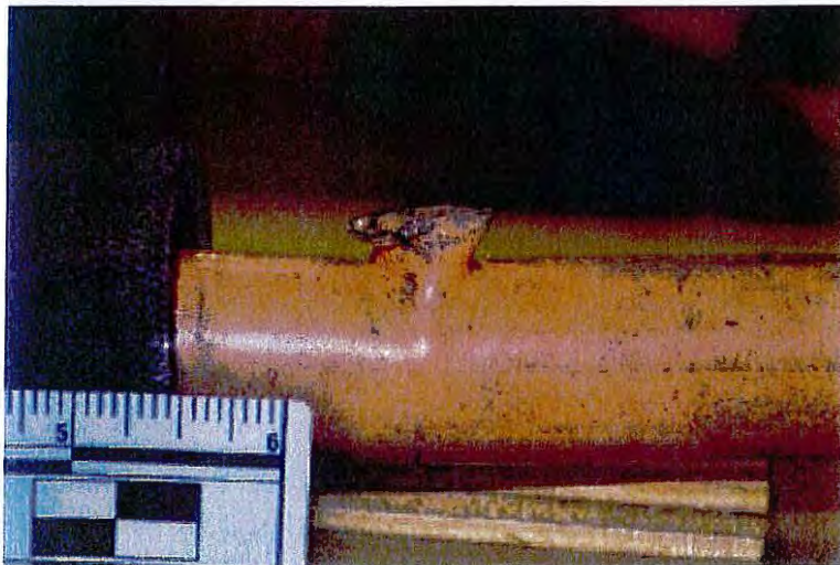
Figure 6: Detail of blowhole. This damage was heat related.
