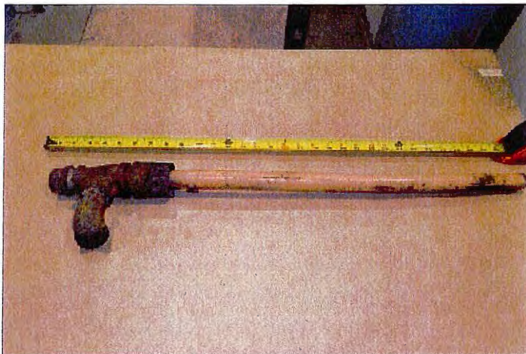
Figure 8: The underside of the foundation fitting assembly and service pipe were unremarkable.
