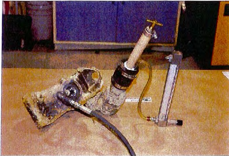
Figure 26: The leak testing apparatus.
