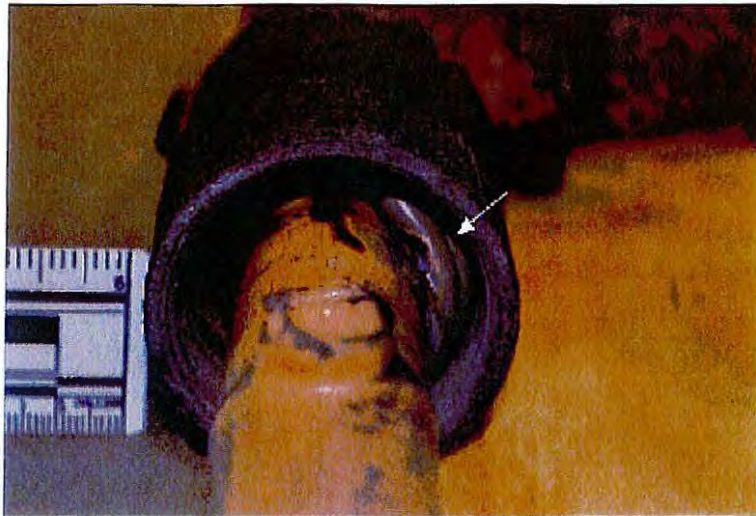
Figure 7: Melted plastic was visible within the foundation fitting, arrow. This was heat related.
