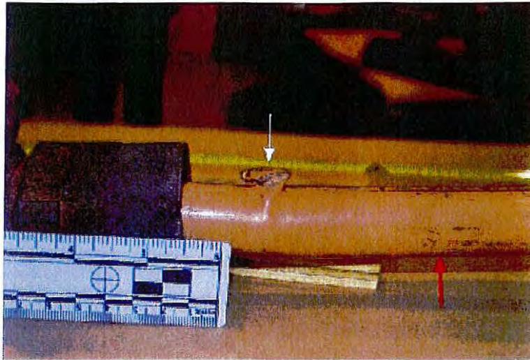
Figure 5: Service line blowhole adjacent to the foundation fitting, white arrow. The service line was bowed on this end, red arrow.
