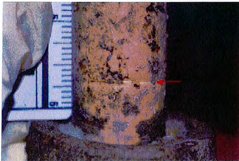
Figure 25: Facing view of saddle pipe dimple, arrow.
