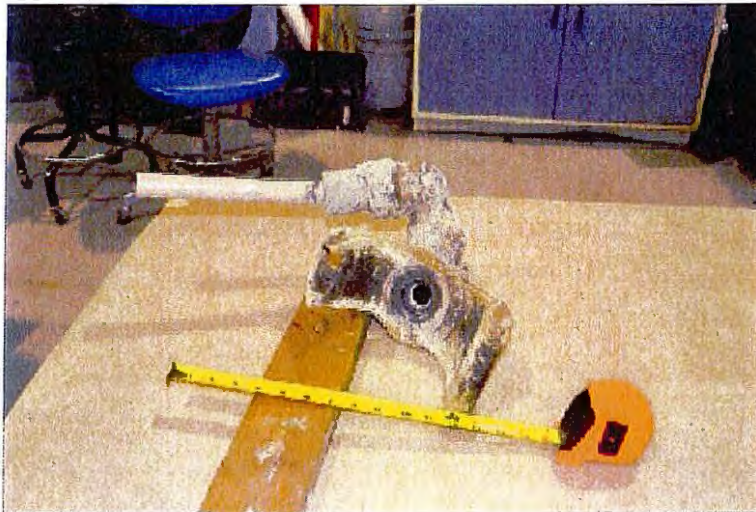
Figure 11: The saddle fitting assembly, bottom view. Note plastic service pipe is askew.
