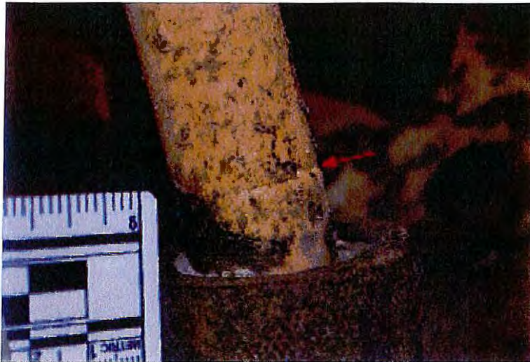
Figure 24: Detail of saddle fitting service pipe after cleaning. Note scrubbed surface texture and dimpled region, arrow.
