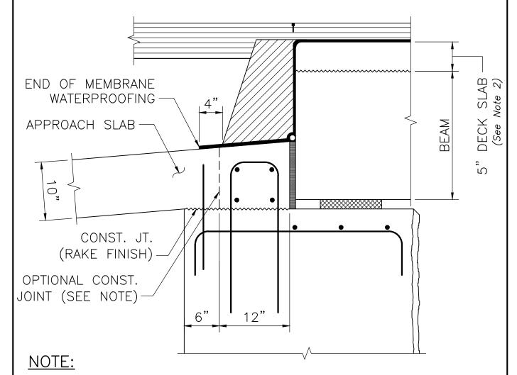
IF THE APPROACH SLAB IS POURED MONOLITHICALLY WITH THE BACKWALLS, MAKE A 2" DEEP BY 1" WIDE SAWCUT IN THE TOP OF THE SLAB AT THE OPTIONAL CONSTRUCTION JOINT LOCATION. FILL SAWCUT WITH CONCRETE JOINT SEALER.
