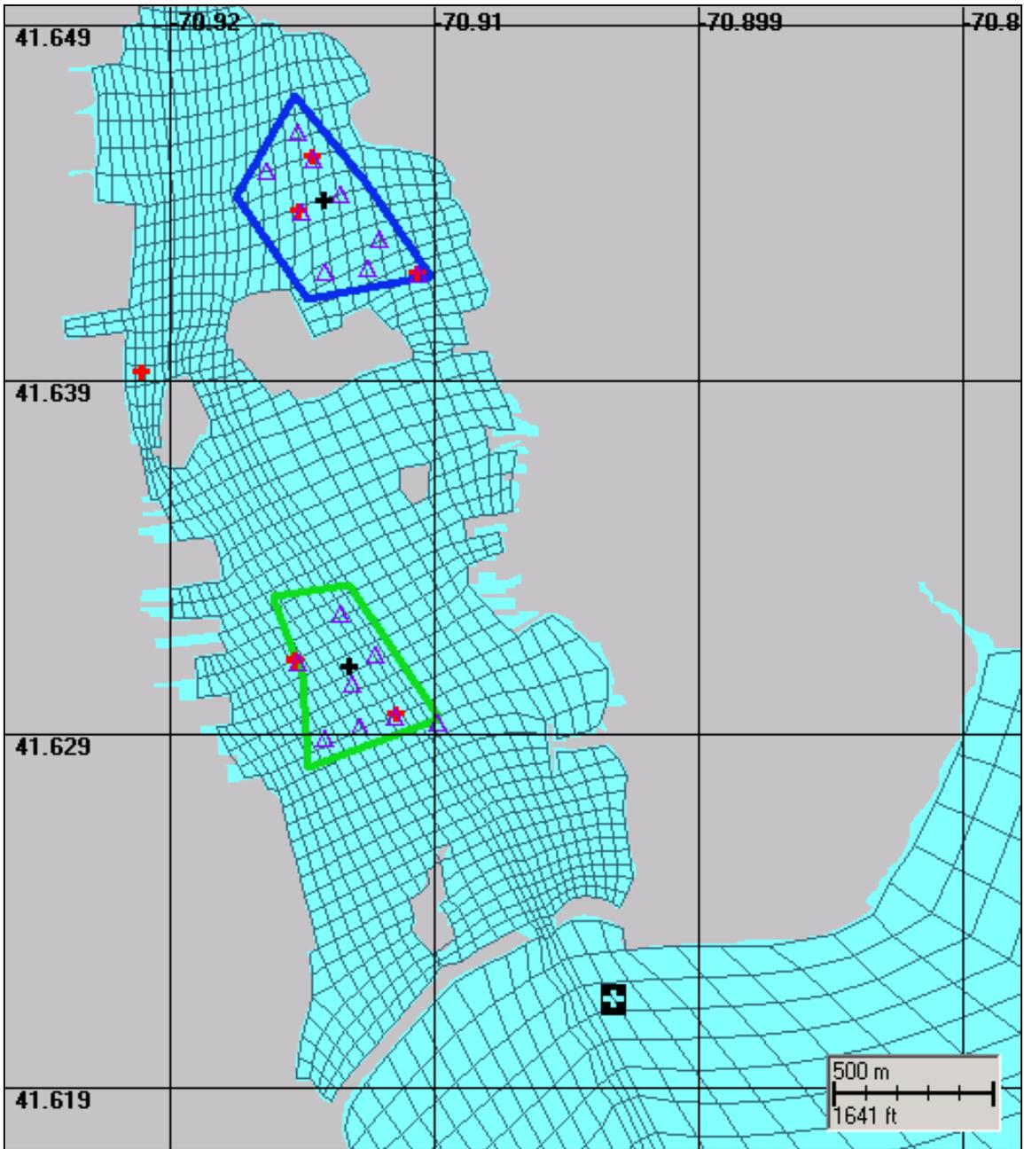
**Figure 2-1. Distribution of two long term deployment stations (black crosses), eleven sediment sampling sites (blue triangles), and six elutriate analyses locations (red crosses). Popes Island (blue polygon) and Channel Inner (green polygon) CAD sites are also shown. Grid of model cells shown is explained in Section 3.**
