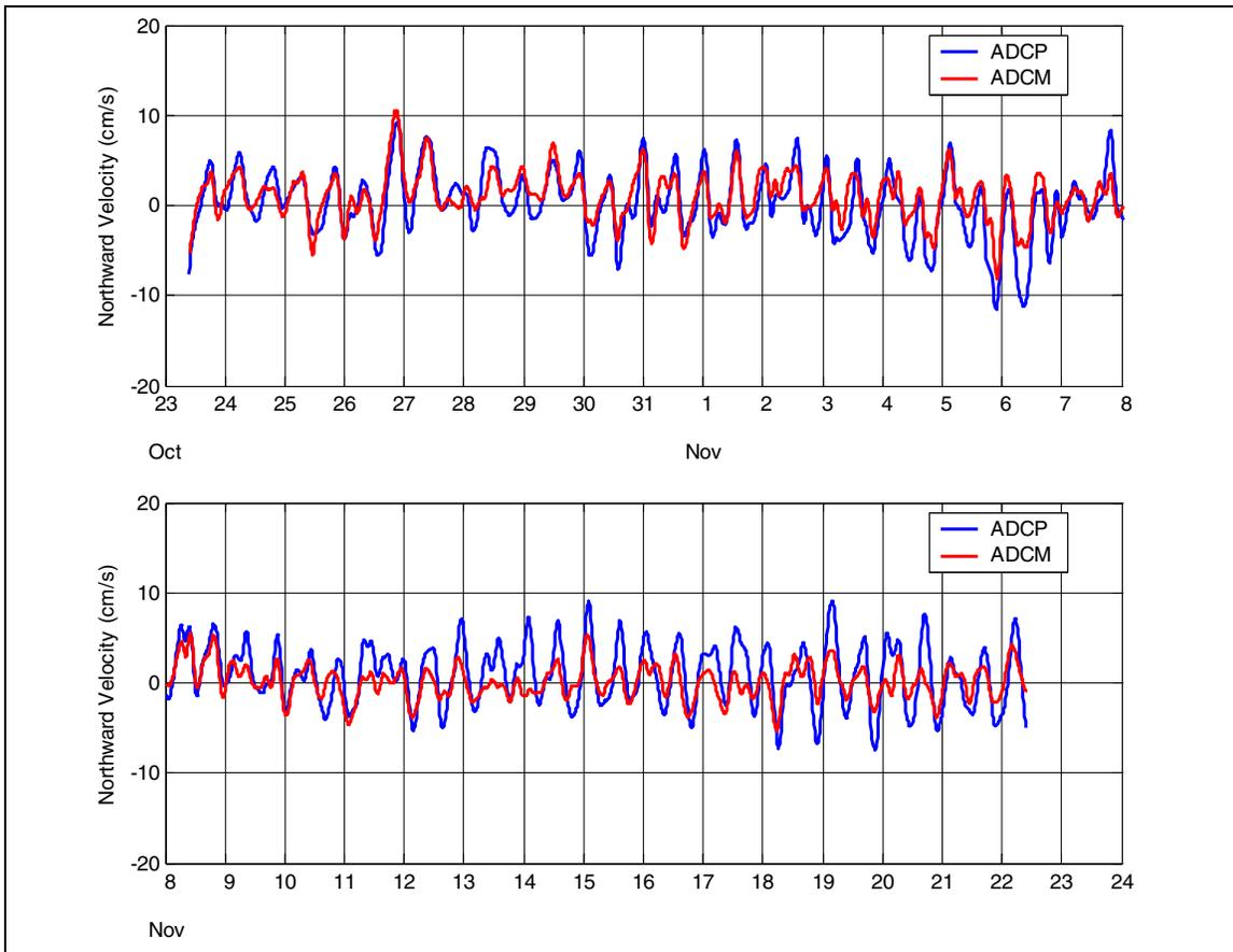
**Figure 2-12. A comparison of the northward component of near bottom current velocity as measured by the ADCP (blue) and the ADCM (red) at the Channel Inner station.**
