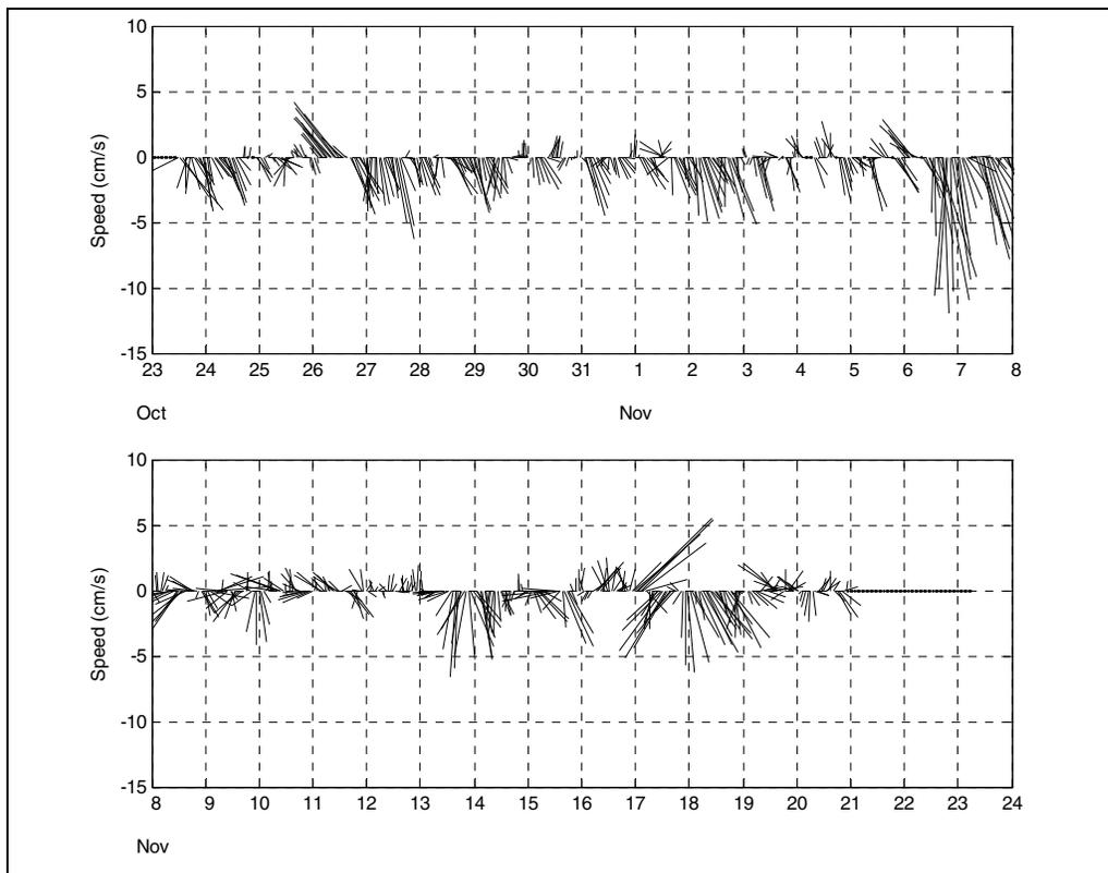
**Figure 2-3. Depth averaged current velocities at the Popes Island station. Individual vectors point in the direction the current is moving to (e.g., a vertical line pointing upwards indicates flow from south to north). The length of each vector is proportional to the current speed. The data have been subsampled at hourly intervals for clarity.**
