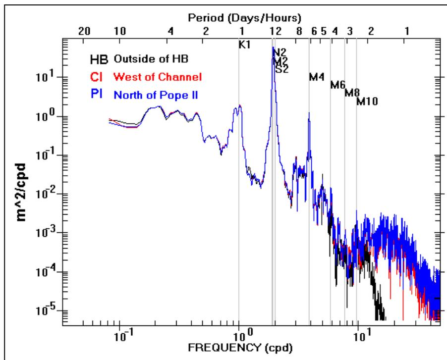
**Figure 3-1. Energy spectrum distribution obtained from surface elevations at the long term deployment stations: HB(Hurricane Barrier), PI (Popes Island north), and CI (Channel Inner). Periods and frequencies of selected tidal constituents are shown.**
