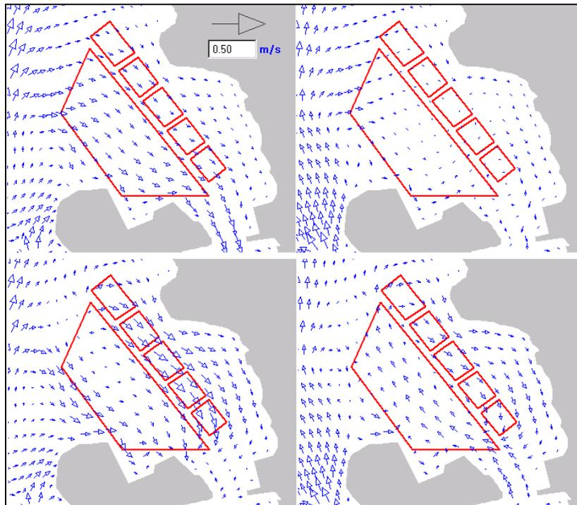
**Figure 3-17 Comparison of velocity vectors at surface (left panels) and bottom (right panels) for the NWW wind case, existing (upper panels) versus excavated (lower panels) bathymetry. Red polygons represent cells in the CAD facility at north of Popes Island.**
