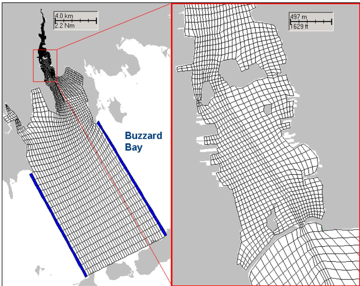
Figure 3-5. New Bedford harbor hydrodynamic model grid
