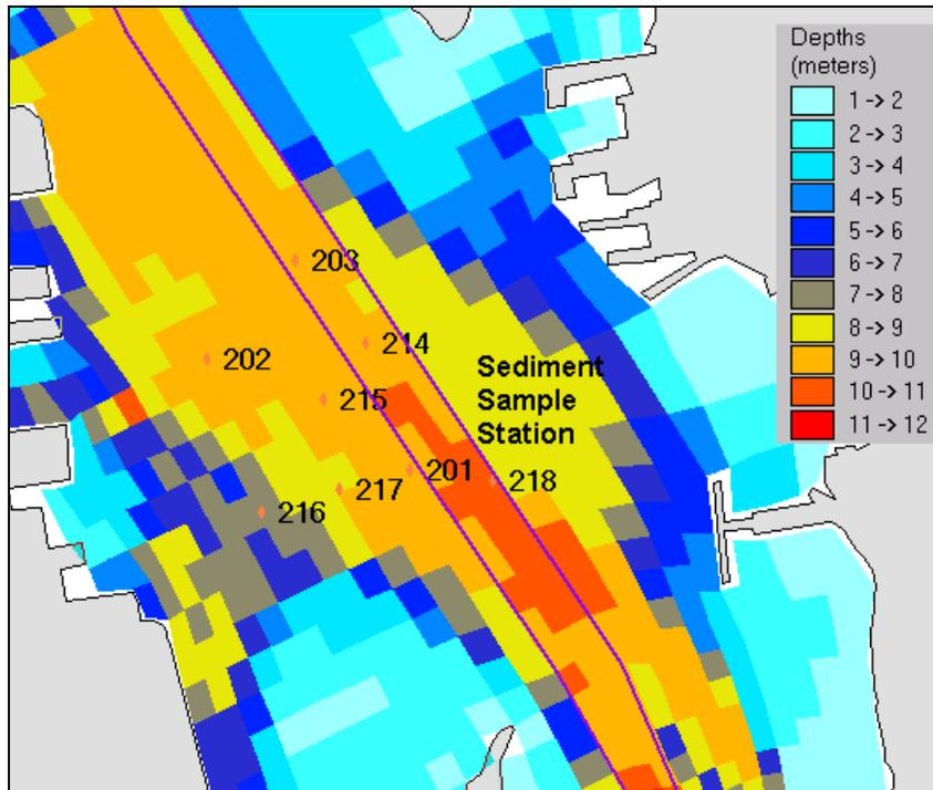
**Figure 4-9. Map showing sediment sampling stations near Channel Inner dredge site.**
