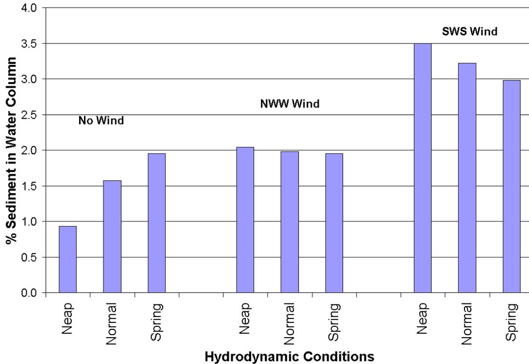
**Figure 4-7 Sediment fractions in water column for various hydrodynamic conditions.**
