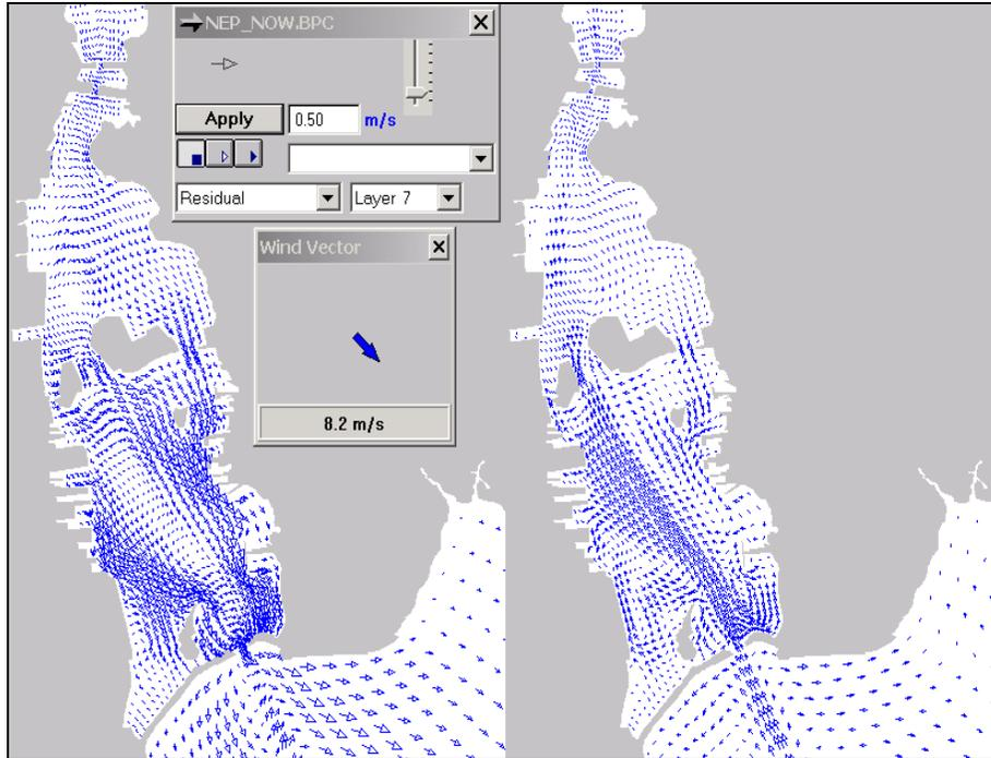
**Figure 3-15. Surface (left) and bottom (right) velocity vectors for NWW wind.**
