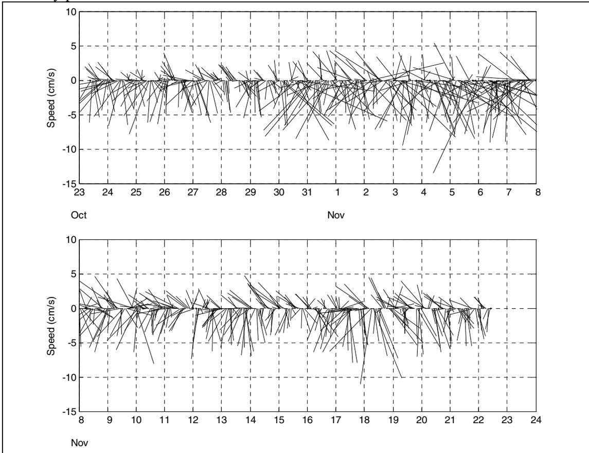
**Figure 2-8. Depth averaged current velocities at the Channel Inner station. Individual vectors point in the direction the current is moving to (e.g., a vertical line pointing upwards indicates flow from south to north). The length of each vector is proportional to the current speed. The data have been subsampled at hourly intervals for clarity.**
