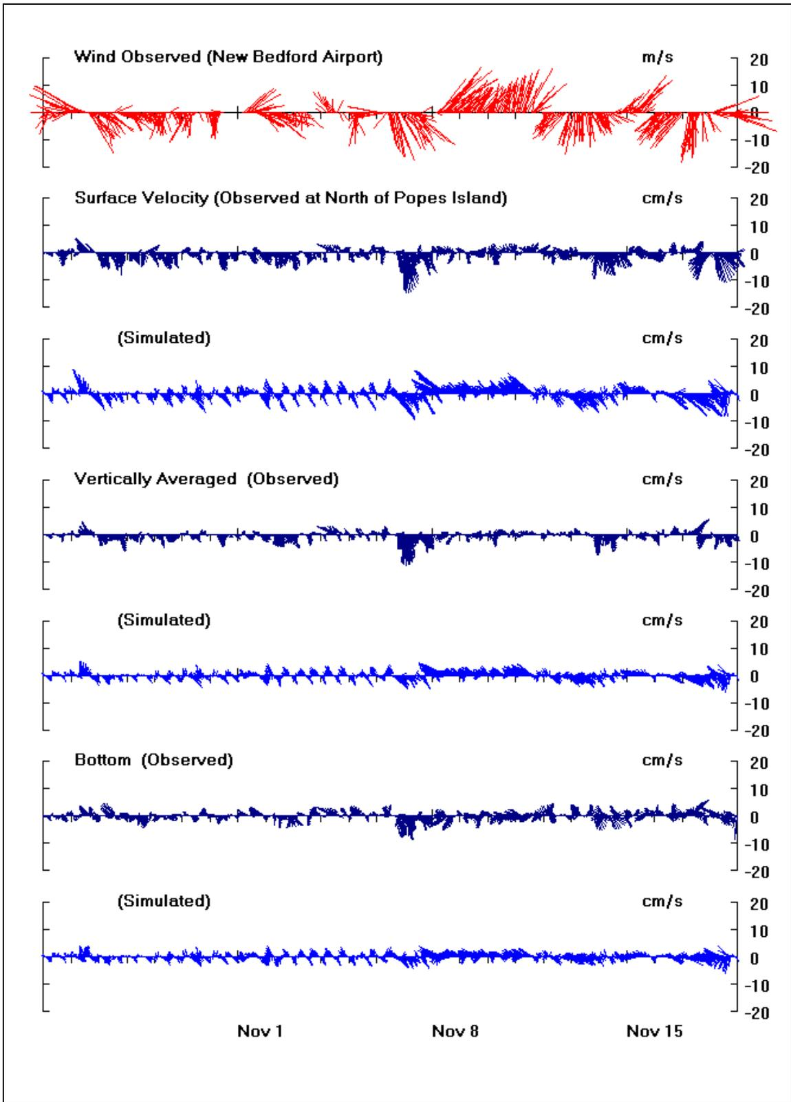
Figure 3-8. Comparison of observed versus simulated velocity at Popes Island north station.
