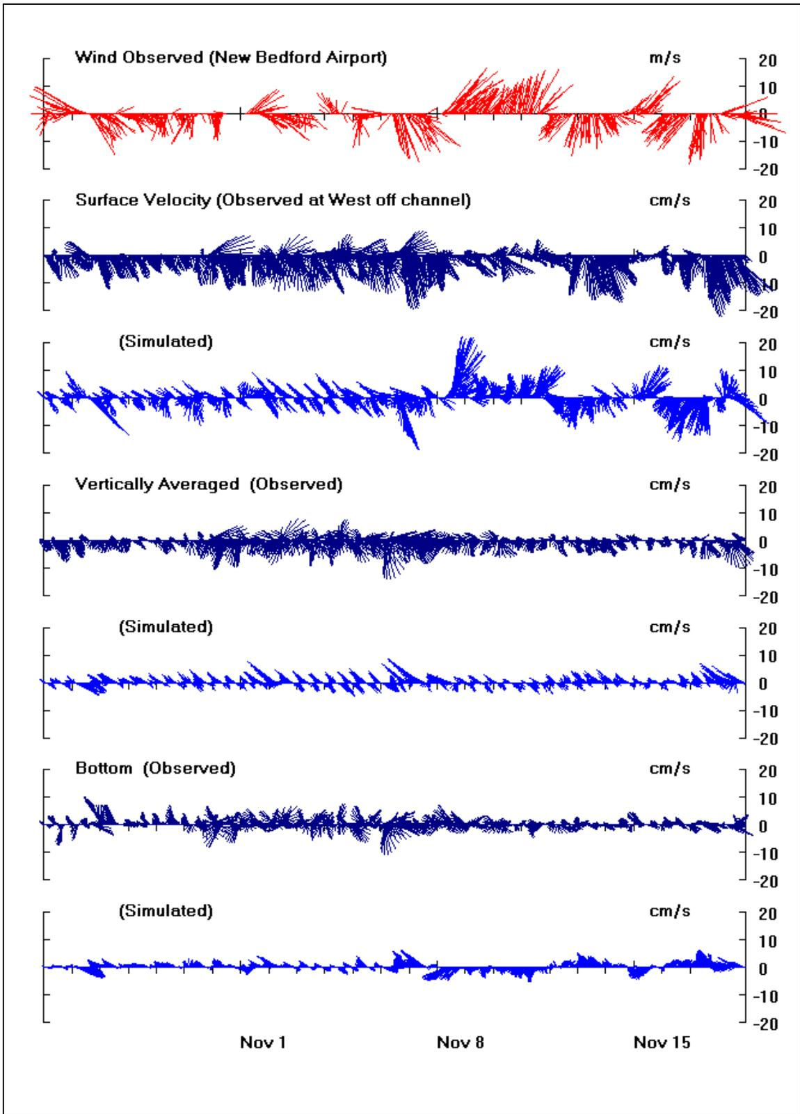
Figure 3-7. Comparison of observed versus simulated velocity at Channel Inner station.
