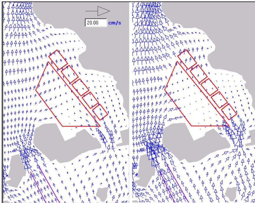
**Figure 3-16 Comparison of flood surface velocity vectors for spring tide and calm winds: existing (left) versus excavated (right) bathymetry. Red polygons represent cells in the proposed CAD facility at north of Popes Island.**
