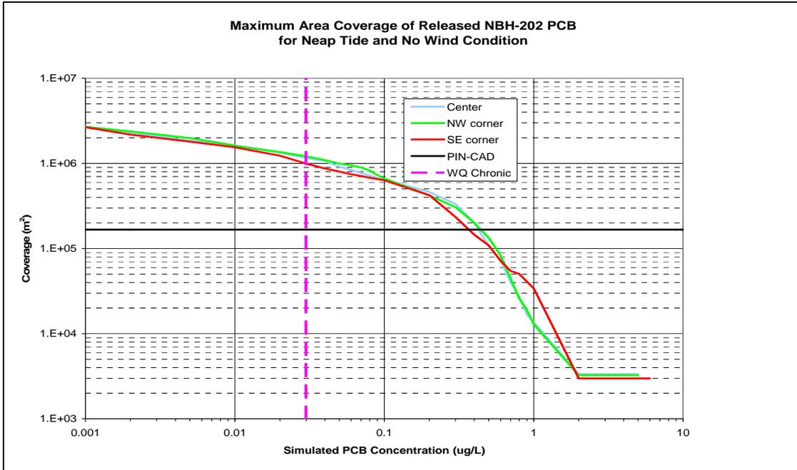
**Figure 5-3. Maximum area coverages (y-axis) of PCBs vs. concentrations for neap tides and calm winds for three release sites using the NBH-202 station source strength. Both x- and y-axes are logarithmic scales. The PIN-CAD cell area ( $1.67 \times 10^5 \text{ m}^2$ ) is shown with a black horizontal line and the U. S. EPA WQ chronic value for PCB ( $0.03 \text{ } \mu\text{g/L}$ ) is shown with a dashed vertical line.**
