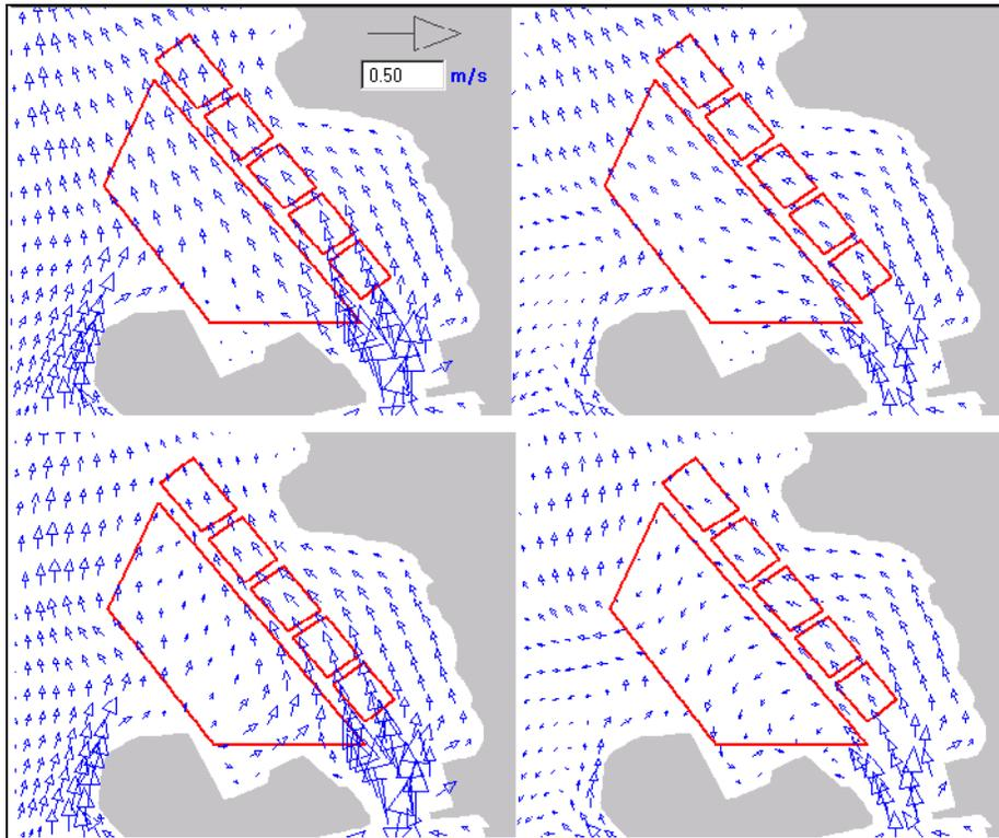
**Figure 3-18 Comparison of velocity vectors at surface (left panels) and bottom (right panels) for the SWS wind case, existing (upper panels) versus excavated (lower panels) bathymetry. Red polygons represent cells in the CAD facility at north of Popes Island.**
