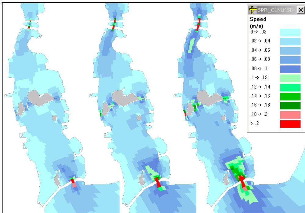
**Figure 3-10. Surface flood speed contours for neap, mean and spring (from left to right) tide conditions under calm wind conditions.**
