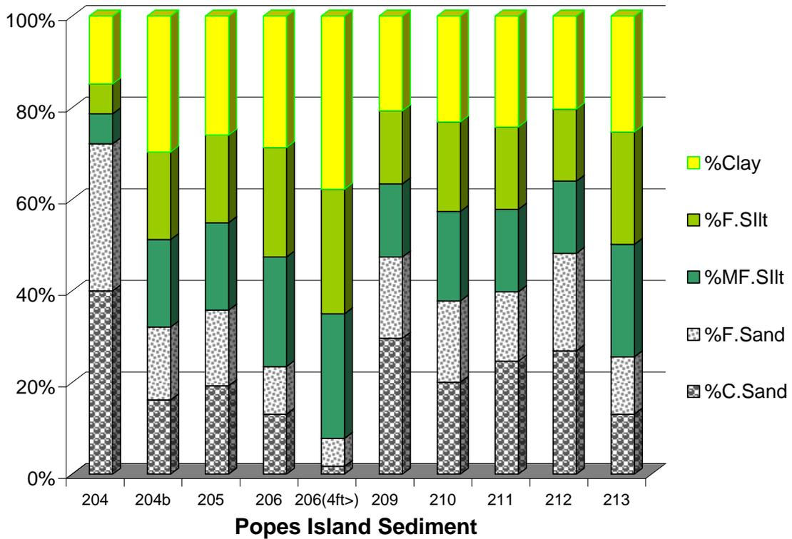
**Figure 4-1 Sediment type distributions near the PIN-CAD cell site.**
