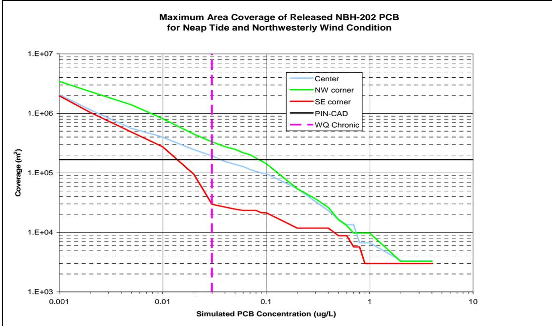
**Figure 5-4. Maximum area coverages (y-axis) of PCBs vs. concentrations for neap tides and northwesterly winds for three release sites using the NBH-202 station source strength. Both x- and y-axis are logarithmic scale. The PIN-CAD cell area ( $1.67 \times 10^5 \text{ m}^2$ ) is shown with a black horizontal line and the U. S. EPA WQ chronic value for PCB ( $0.03 \text{ } \mu\text{g/L}$ ) is shown with a dashed vertical line.**
