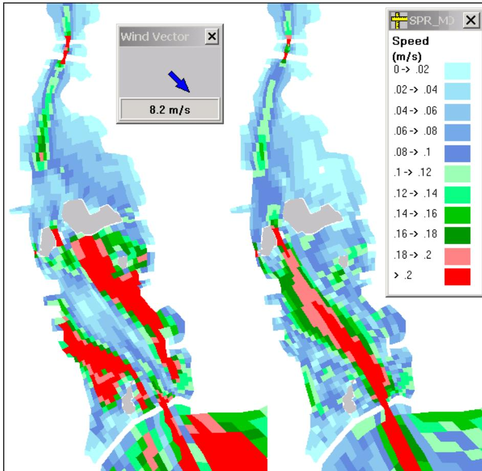
Figure 3-14. Surface (left) and bottom (right) speed contours for NWW wind.
