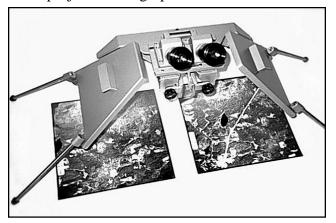
Figure 2: Mirror stereoscope
