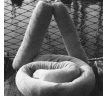
Absorption booms are effective for controlling small spills.
