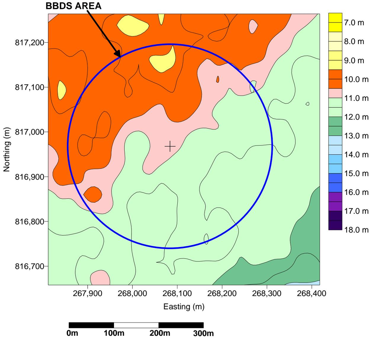
**Figure 3-3.** Bathymetric results from the BBDS Survey Area (NAD 83), contour interval = 0.2 m.
