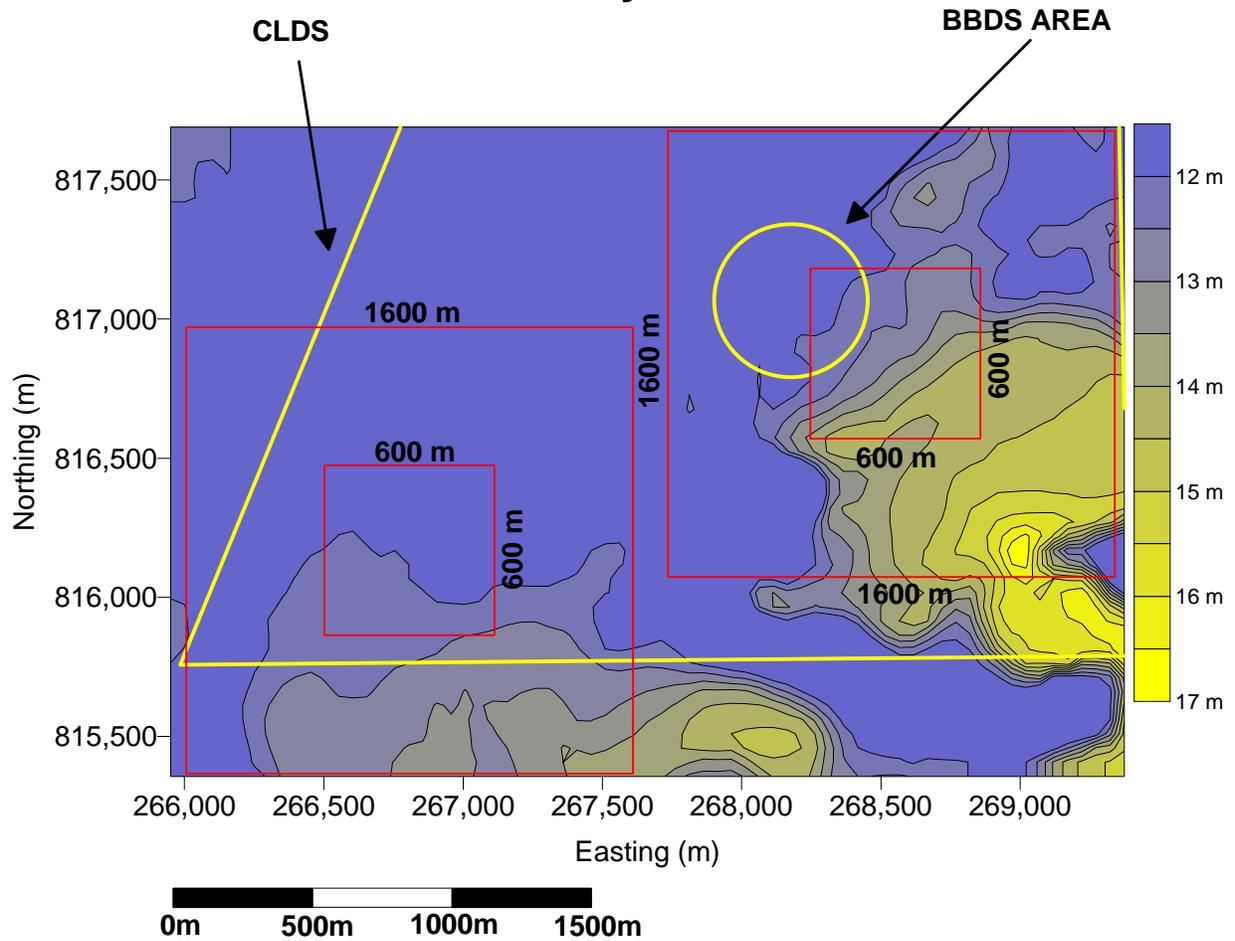
**Figure 4-1.** Bathymetry of the Cleveland Ledge Survey Area highlighting water depths of greater than 12 m.
