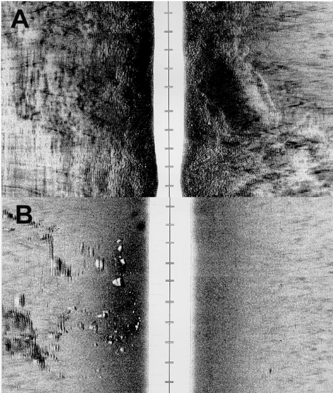
**Figure 2-2.** Examples of rocky bottom texture from side-scan data including (A) rock ledge (Giffords Ledge) and (B) scattered rocks.
