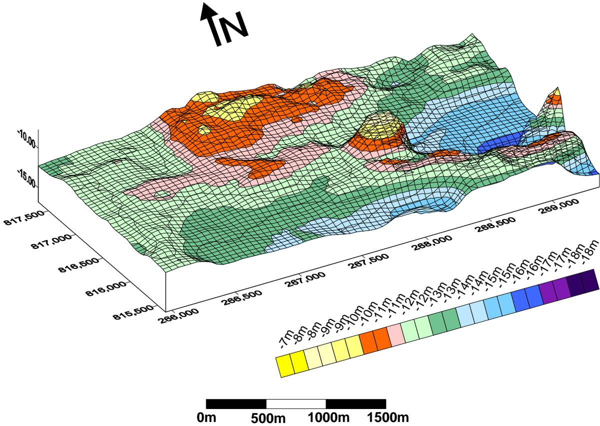
Figure 3-2. Three-dimensional view of the Cleveland Ledge Survey Area bathymetry.
