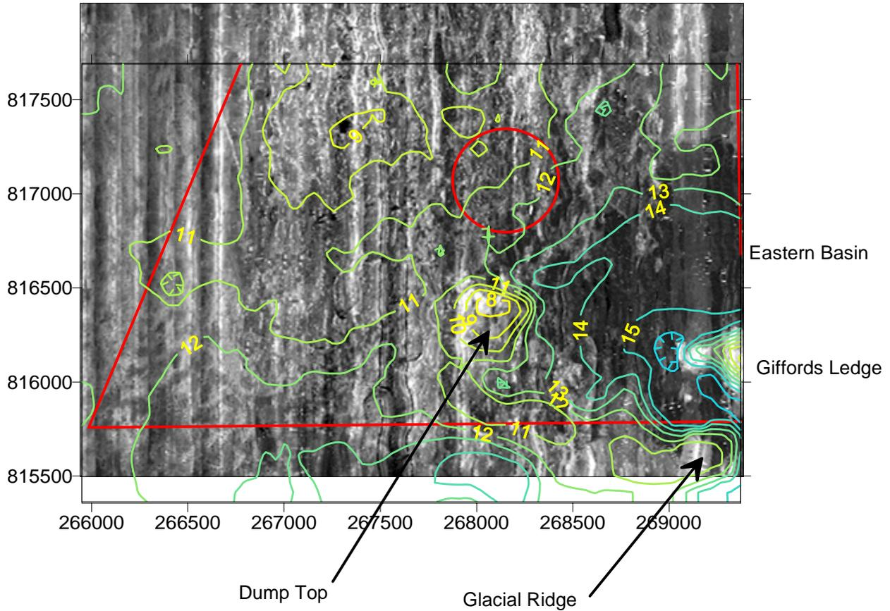
**Figure 3-7.** Side-scan mosaic of the Cleveland Ledge Survey Area overlaid by approximate location of bottom contours.
