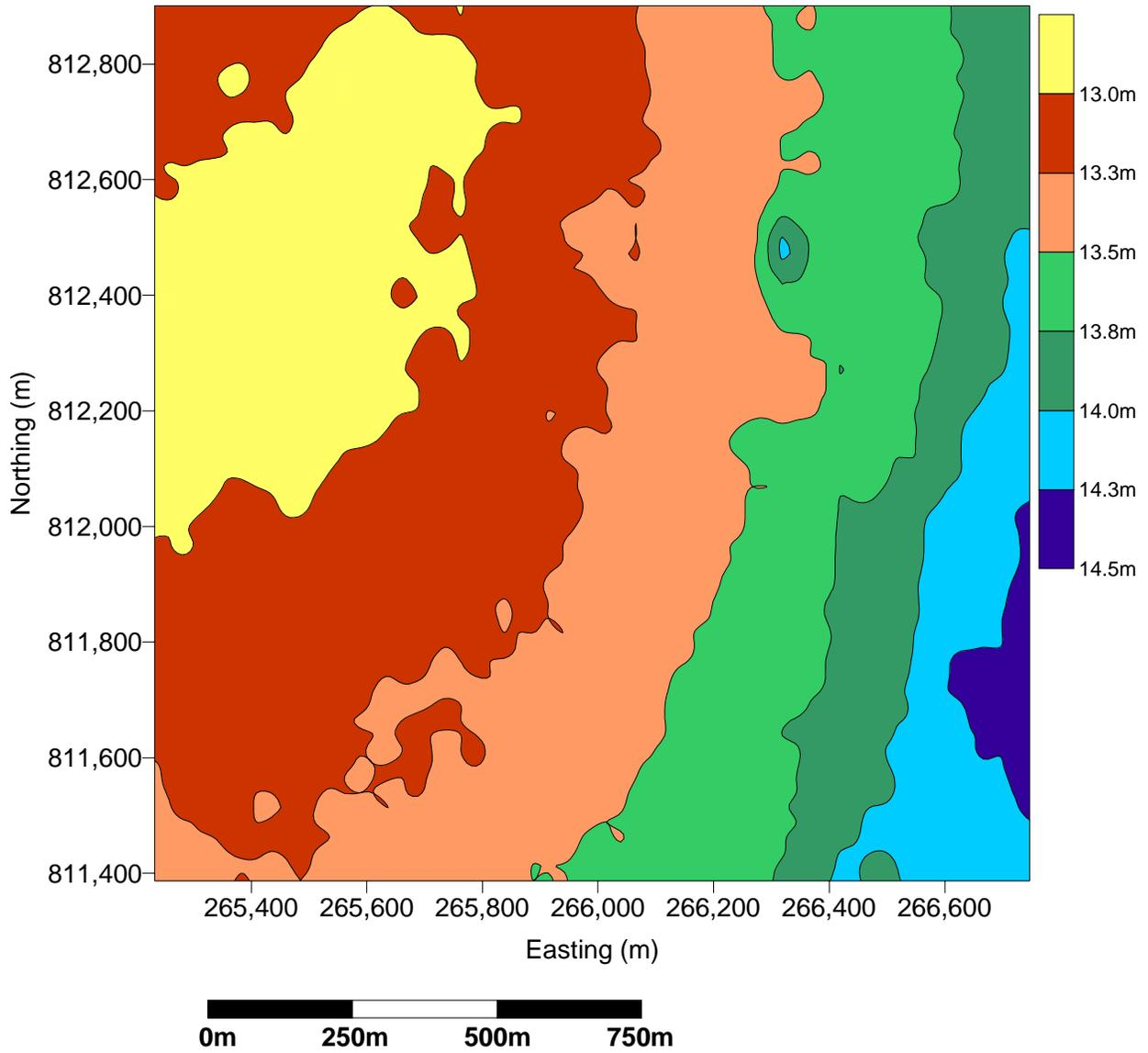
**Figure 3-5.** Bathymetric results from the Quisset Survey Area (NAD 83), contour interval = 0.2 m.
