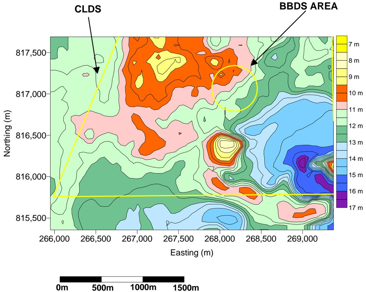
**Figure 3-1.** Bathymetric results from the Cleveland Ledge Survey Area (NAD 83), contour interval = 0.5 m.
