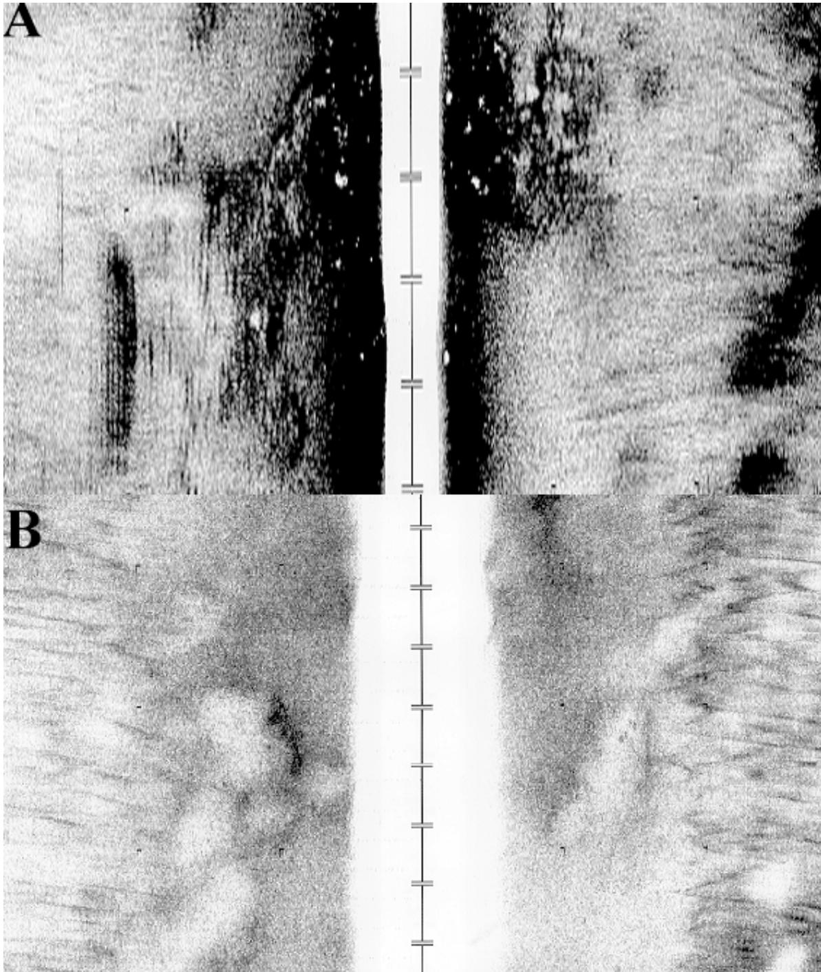
**Figure 2-1.** Examples of the acoustic appearance of dredged material, including (A) rubbled texture and (B) cratered texture.
