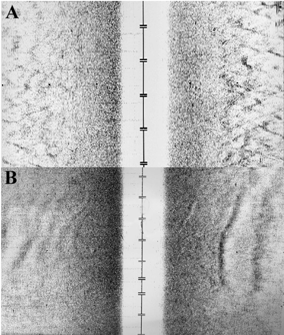
**Figure 2-3.** Examples of bottom textures from side-scan data showing (A) ambient bottom and (B) sand waves.
