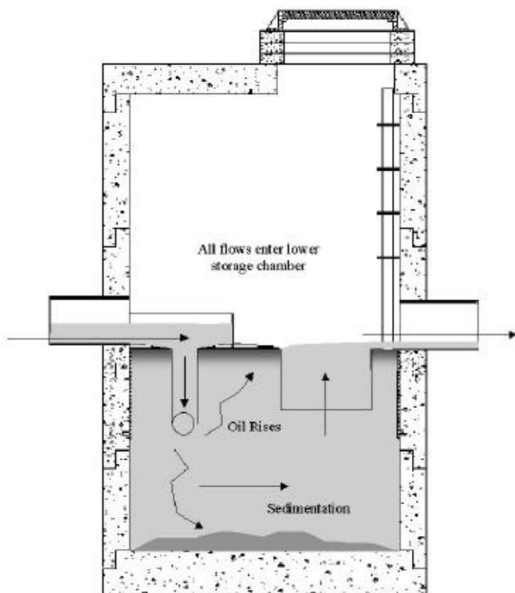
Figure 2. Stormceptor operation during average flow conditions.
