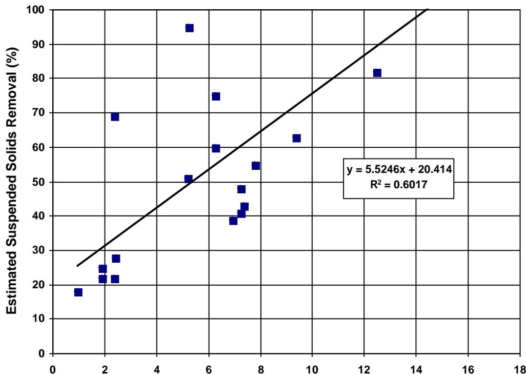
Figure 3: Stormceptor® Sizing Guideline - Removal efficiency as a function of storage capacity from 23 Stormceptor units in Toronto Canada.
