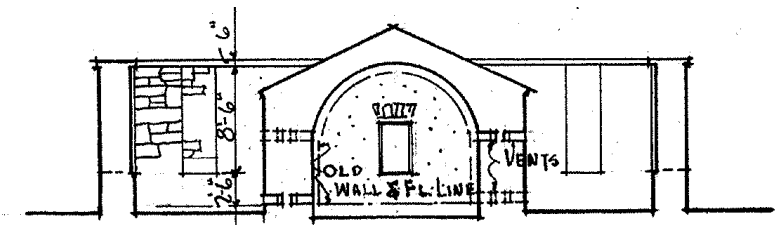
5.6: Cross section of the Pikesville Magazine and its wall. Like the Captain's Island magazine, it had roof of slates over common rafters. It also had a system of narrow indirect vents through the walls.
