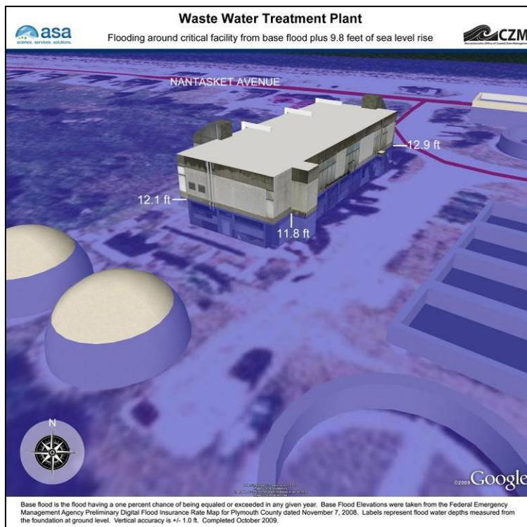
**Figure A-20. Waste Water Pollution Control Facility, View 2, Base Flood Elevation plus 9.8 feet of sea level rise.**
