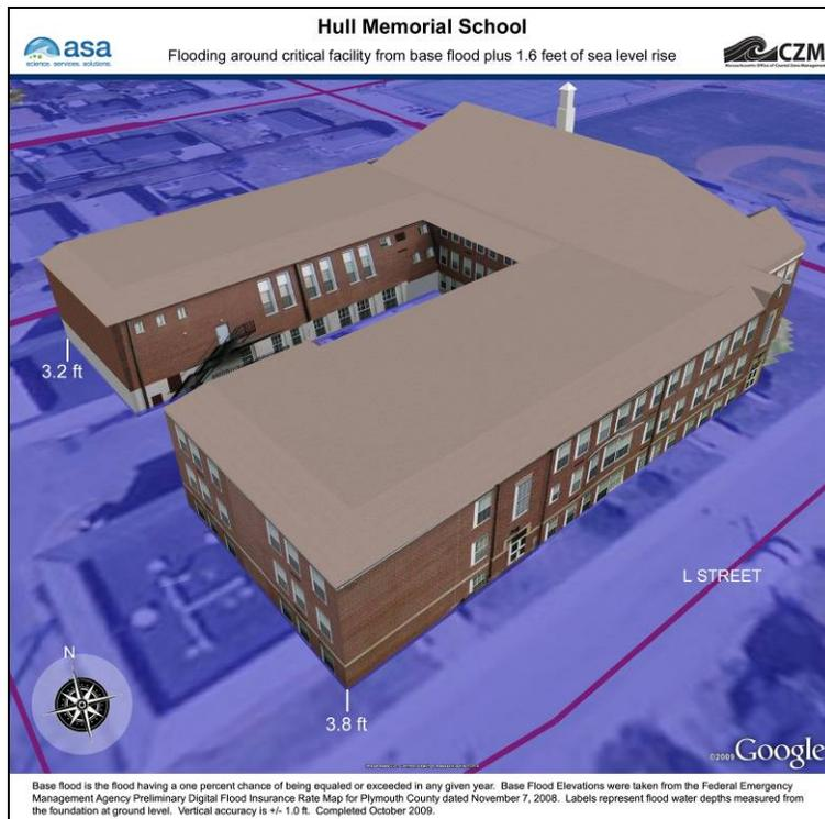
**Figure A-58. Hull Memorial School, View 2, Base Flood Elevation plus 1.6 feet of sea level rise.**
