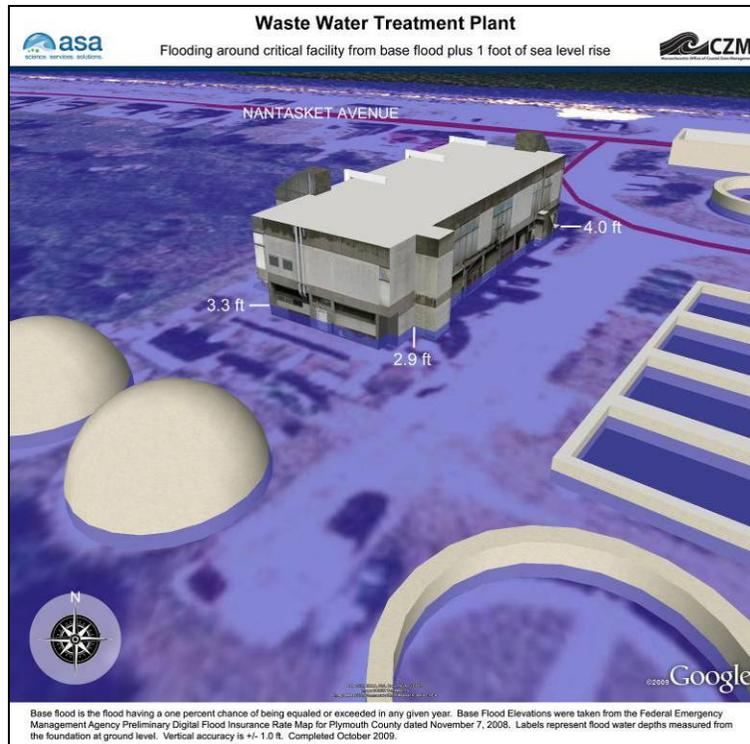
**Figure A-17. Waste Water Pollution Control Facility, View 2, Base Flood Elevation plus 1 foot of sea level rise.**
