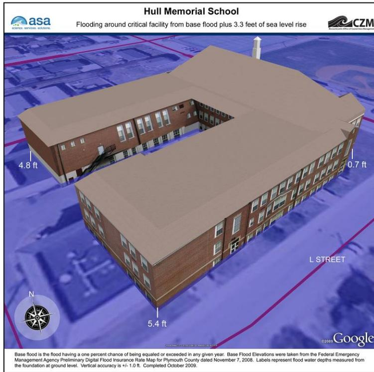
Figure A-59. Hull Memorial School, View 2, Base Flood Elevation plus 3.3 feet of sea level rise.
