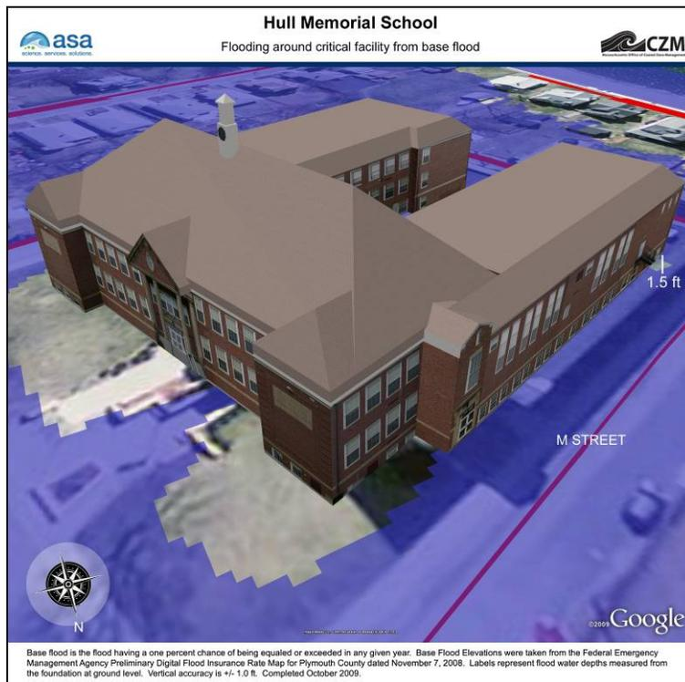
**Figure A-51. Hull Memorial School, View 1, Base Flood Elevation.**
