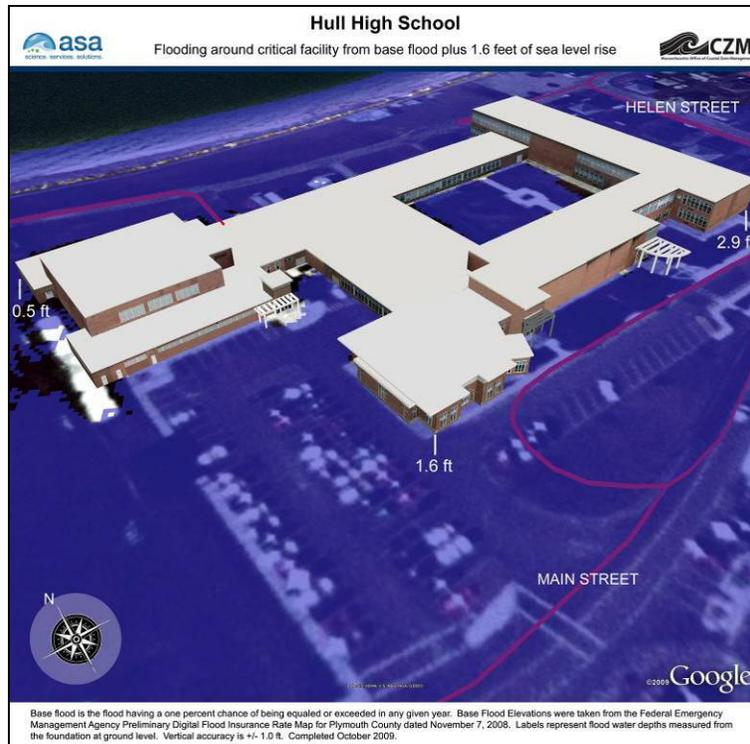
Figure A-23. Hull High School, View 1, Base Flood Elevation plus 1.6 feet of sea level rise.
