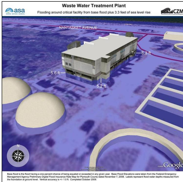
**Figure A-19. Waste Water Pollution Control Facility, View 2, Base Flood Elevation plus 3.3 feet of sea level rise.**
