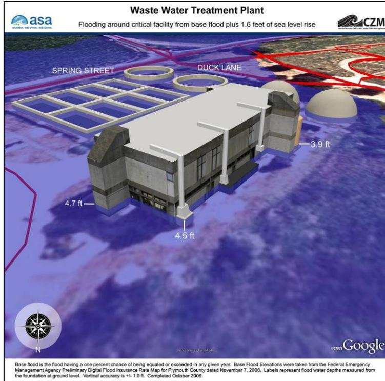
**Figure A-13. Waste Water Pollution Control Facility, View 1, Base Flood Elevation plus 1.6 feet of sea level rise.**
