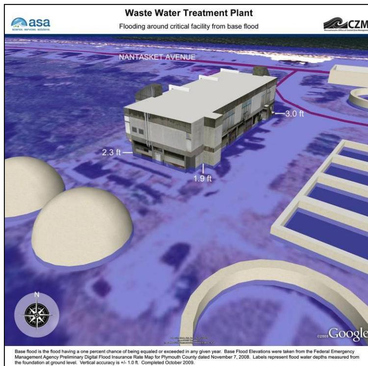
**Figure A-16. Waste Water Pollution Control Facility, View 2, Base Flood Elevation.**
