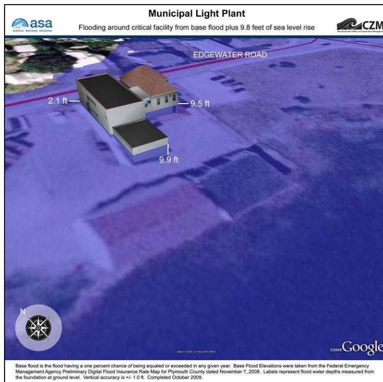
Figure A-40. Municipal Light Plant, View 2, Base Flood Elevation plus 9.8 feet of sea level rise.
