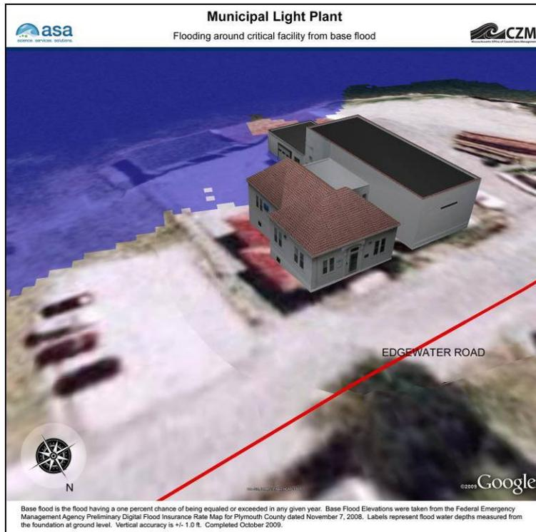
**Figure A-31. Municipal Light Plant, View 1, Base Flood Elevation.**
