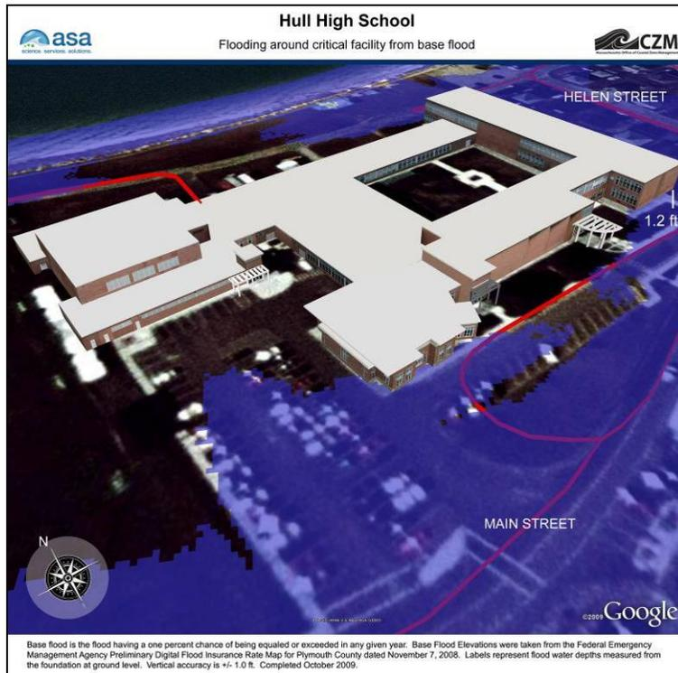
Figure A-21. Hull High School, View 1, Base Flood Elevation.
