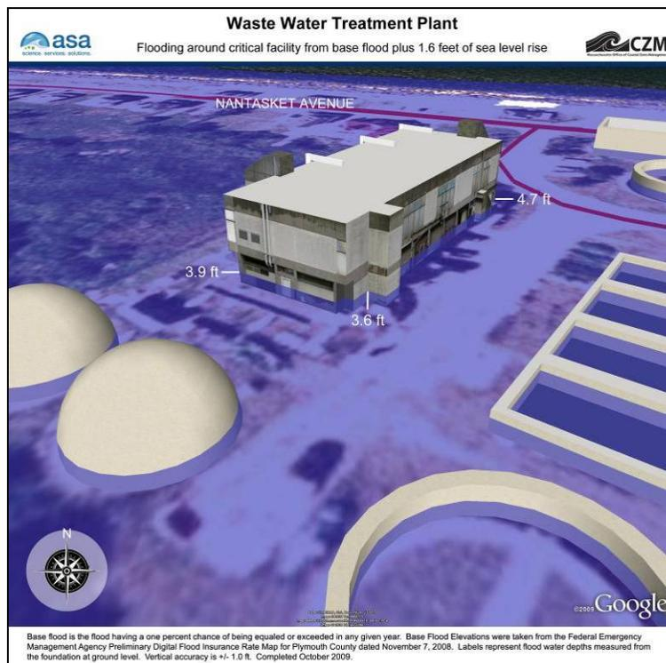
**Figure A-18. Waste Water Pollution Control Facility, View 2, Base Flood Elevation plus 1.6 feet of sea level rise.**
