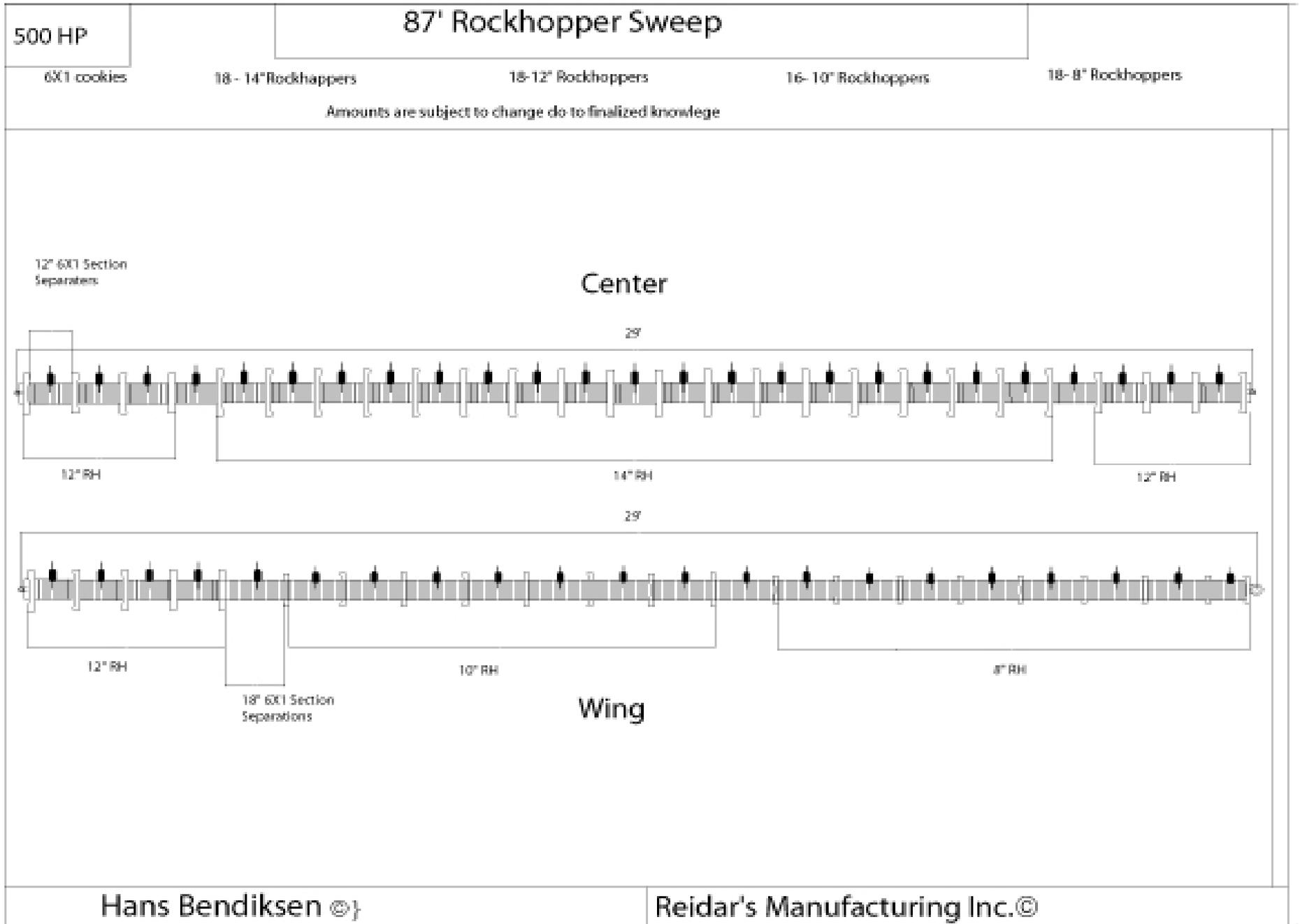
Sweep schematic and tri-plate detail
