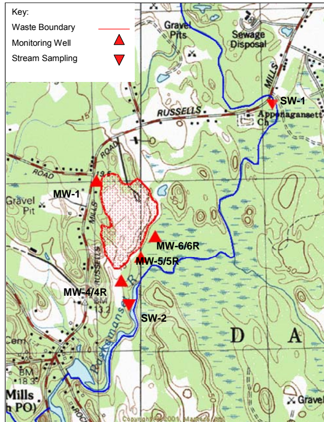
Figure IV-5. Town of Dartmouth landfill site. The estimated landfill material is denoted by the red line. Groundwater monitoring wells are located both up-gradient (MW-1) and down-gradient (MW-4, 5, 6). SW-1 and SW-2 are stream monitoring sites on the Paskamanset River. The wells and stream sites have been monitored twice a year since about 1995. Landfill was capped in 1996.
