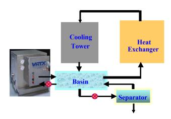
and returned back to the tower basin. The water discharge from the VRTX unit is returned to the basin and a second side-stream taken from the bottom of the cooling tower basin passes through a cyclonic separator or filtration system where the solid calcium carbonate precipitate and other incidental solids can be easily separated from the water and collected. The collected solids are backflushed or siphoned from the system daily.
