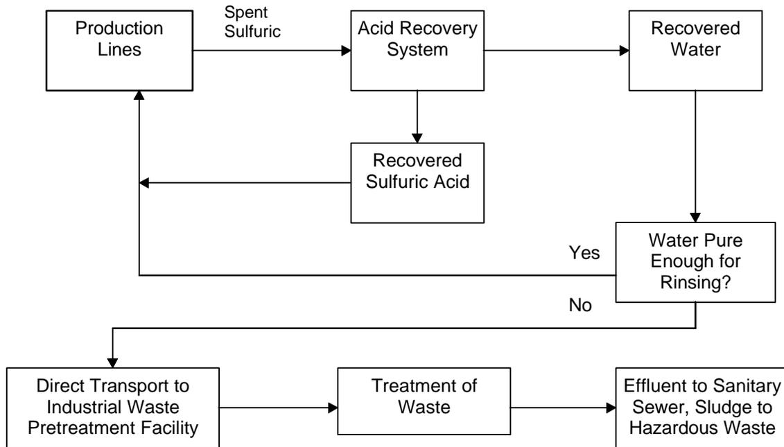
Figure 2 shows the process as modified by the Acid Recovery System. Hazardous material is transferred automatically with pumps from the process to the recovery system. The reject stream is the only component which would require handling if it is not pure enough to be used as a rinse and less handling means less potential exposure.
