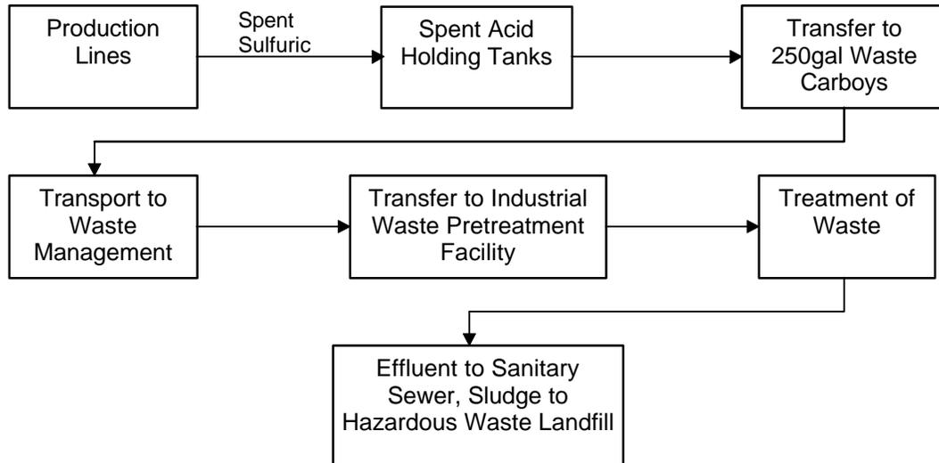
As shown in Figure 1, the spent sulfuric is transferred several times before ultimately being treated and disposed. Transfers and transportation could potentially cause worker exposure to hazardous material via spills or splashes. In addition, none of the acid is reusable and must be treated with additional chemicals and resources.
