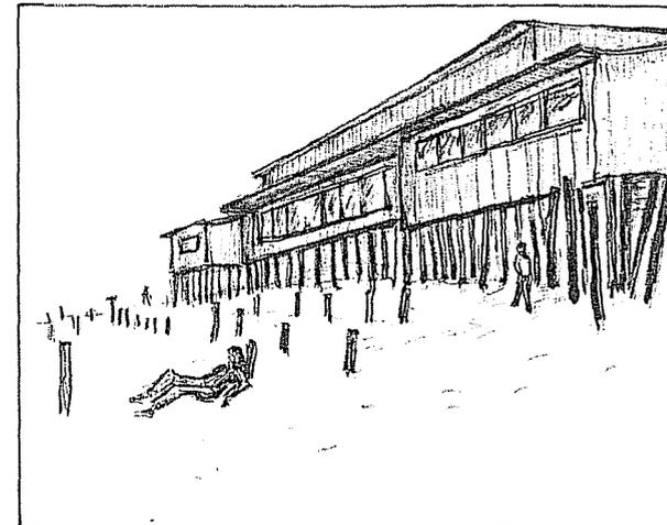
Pilings are made from treated wood poles, concrete or steel. Piles are driven or placed in holes in the substrate.
