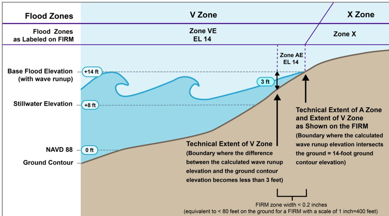
**Figure 5.** Cross-sectional diagram of flood zones on a steep embankment with runup. Here, an A Zone is shown in the profile, but would not be mapped on the FIRM because the zone is less than 0.2 inches in width on the FIRM—thereby not meeting the minimum zone width for mapping at the scale used for FIRMs. Where A Zones such as these are not mapped, the V Zone will extend to the designated ground elevation that corresponds to the V Zone BFE on the FIRM.
