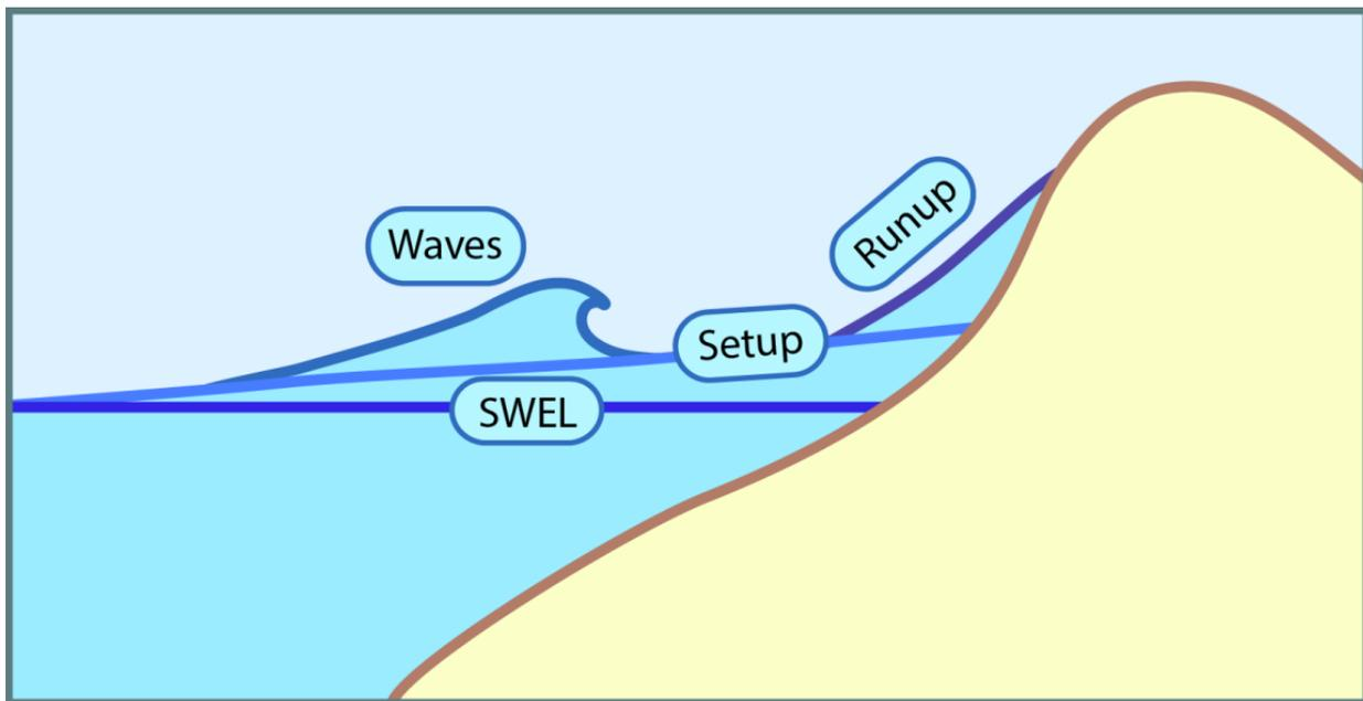
**Figure 2.** The coastal storm surge stillwater elevation (i.e., the line labeled SWEL on the figure) and the added effects of wave setup and wave runup. Figure modified from FEMA Region II Coastal Analysis and Mapping website ([www.region2coastal.com/coastal-mapping-basics](http://www.region2coastal.com/coastal-mapping-basics)).
