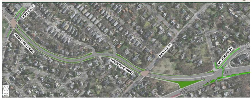
Option B for Fresh Pond Parkway between Huron and Mount Auburn includes many of the same elements as Option A (listed above). The differences are as follows: raised table intersections at Huron and Brattle; floating eastbound bicycle lane rather than signal protected bicycle lane on Huron (meaning the lane is located between turning and through movement vehicle lanes); and configuration change at Larch Road eliminating right turns onto Fresh Pond Parkway.
