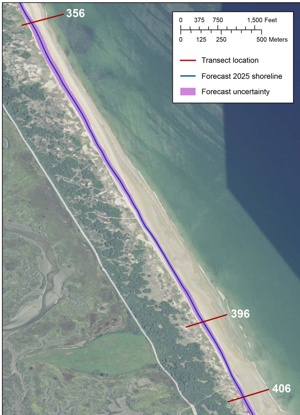
Figure 11. Map showing three example transects and alongshore variability of forecast shoreline position for a portion of Plum Island, Massachusetts using a Kalman filter approach. The transects are shown in greater detail in figures 3-5.
