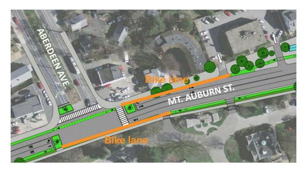
It is imperative that the bike facilities on Mt. Auburn St be continuous, for both safety and comfort of all road users. The short gap in bike lanes in both directions on Mt. Auburn St at
