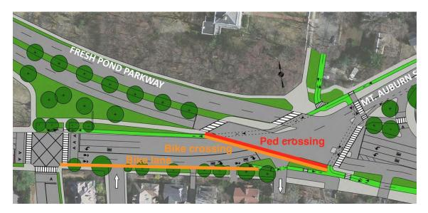
A few critical gaps for pedestrians and bicyclists exist in the current plans for the Mt. Auburn St/Fresh Point Parkway intersection. The largest gap is on the west side of the intersection. Pedestrians and bicyclists traveling along the west side of the parkway would be required to cross three legs of the intersection rather than one, resulting in significant inconvenience and delay. Many will simply follow the desire line and cross where no crossings are provided.
