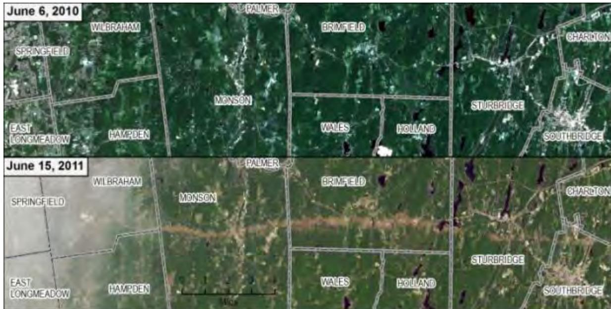
**Figure 1.4** – Landsat 5 Thematic Mapper scenes showing tornado damage (8,500 acres) in western Massachusetts. Data source: USGS GLOVIS.
