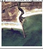
Figure 2. An inlet channel with a jetty on one side and a natural feature on the opposite side, creating a diagonal inlet.
