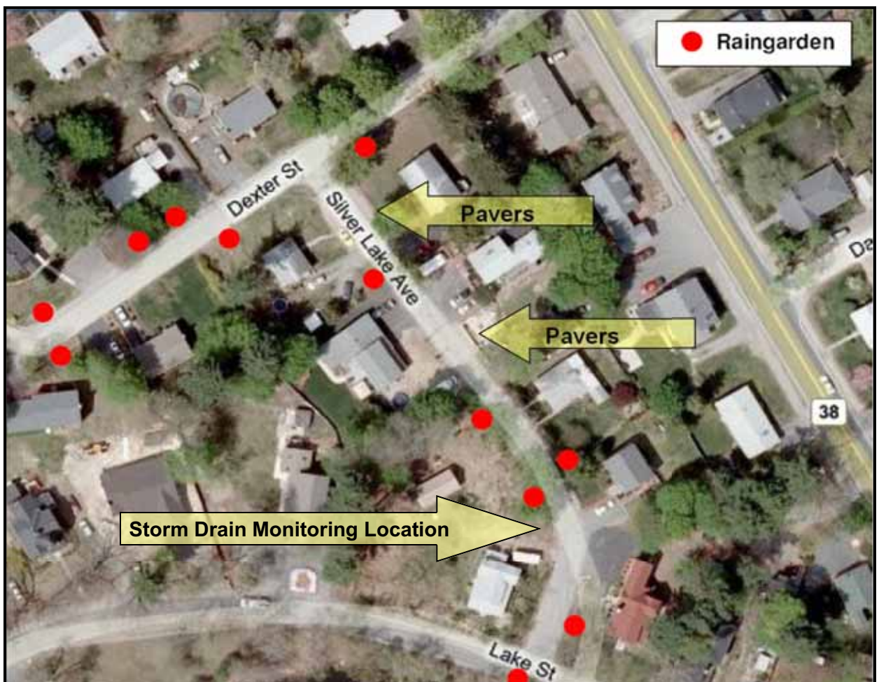
Location of LID features and the monitoring site in the Silver Lake neighborhood
