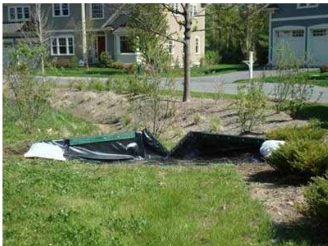
Water was measured as it passed through V-notched weirs (pictured) and other structures.
