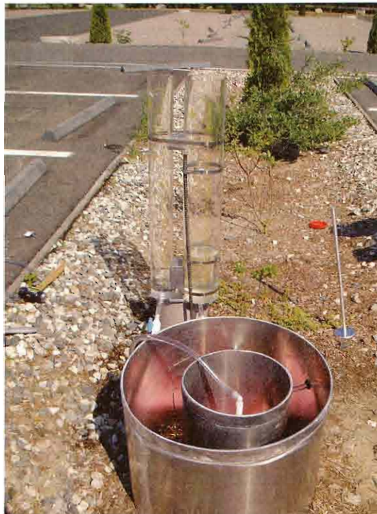
Because of their ability to directly measure vertical flow into the soil, single-ring and double-ring infiltrometer tests were used to assess surface infiltration rates on two bioretention cells, one rain garden, and all four porous pavement surfaces at the project site.
