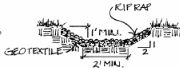
Riprap conveyance channel profile
