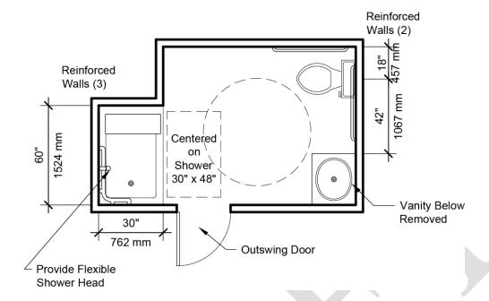
b. All walls of the shower shall have structural reinforcement to allow the future installation of a seat and grab bars, at any location from the floor to a height of 60 inches (1524 mm) above the floor.
