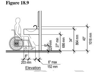
d. A *clear floor space* complying with **521 CMR 7.00: GROUND AND FLOOR SURFACES** and positioned for a forward approach, and knee and toe clearance complying with **521 CMR 6.3, Knee Clearance**, and **521 CMR 6.4 Toe Clearance** shall be provided.
