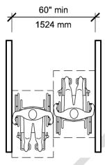
8.5.1 An *accessible route* with a *clear* width less than 60 inches (1524 mm) shall provide a passing space at intervals of 200 feet (60960 mm) maximum. Passing spaces shall be either: a space 60 inches by 60 inches (1524 mm by 1524 mm) minimum; or, an intersection of two (2) walking surfaces providing a T-shaped space complying with **521 CMR 6.2.1** where the base and arms of the T-shaped space extend 48 inches (1219 mm) minimum beyond the intersection. See **Figures 8.5b and 8.5c**.
