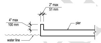
3. In existing piers, *clear* pier space shall be permitted to be located perpendicular to the *boat slip* and shall extend the width of the *boat slip*, where the *facility* has at least one (1) *boat slip* complying with **521 CMR 60.5**, **Clearances**, and further compliance with **521 CMR 60.5**, **Clearances**, would result in a reduction in the number of *boat slips* available or result in a reduction of the widths of existing slips. See **Figure 60.5c**.
