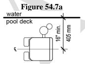
c. On the side of the seat opposite the water, a *clear* deck space shall be provided parallel with the seat. The space shall be 36 inches (914 mm) wide minimum and shall extend forward 48 inches (1219 mm) minimum from a line located 12 inches (305 mm) behind the rear edge of the seat. The *clear* deck space shall have a slope not steeper than one-to-forty-eight (1:48) (2 percent). See **Figure 54.7b**.
