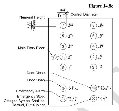
d. The control button for the emergency stop, alarm, door open, door close, main entry floor, and phone, shall be identified with *tactile* symbols as shown in **Figure 14.8c** and **Figure 14.8d**.
