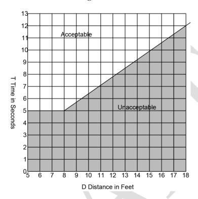
For cars with in-car lanterns, "T" begins when the lantern is visible from the vicinity of hall call buttons and an audible signal is sounded.
