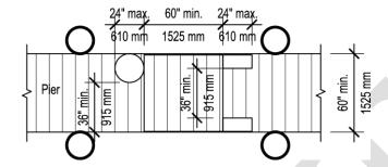
2. Edge protection shall be permitted at the continuous *clear* openings, provided that it is 4 inches (102 mm) high maximum and 2 inches (51 mm) wide maximum. See **Figure 60.5b**.
