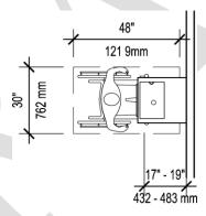
17.2.2 Free-standing units not having a knee clearance under them shall have a *clear floor or ground space* that allows a person in a wheelchair to make a parallel approach to the unit. See **Figure 17.2d**. This *clear floor or ground space* shall comply with **521 CMR 6.6**, **Side Reach**.
