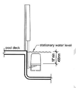
Pool Lift Submerged Depth Figure 54.6
