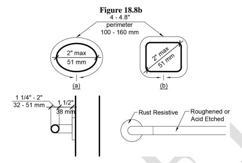
h. Grab bars shall also be non-rusting and acid-etched or roughened. Grab bars shall comply with the *structural strength* defined in **521 CMR 5.00: DEFINITIONS.**
