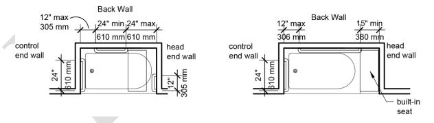
19.9.4 Controls, other than drain stoppers, shall be located on an end wall. Controls shall be between the bathtub rim and grab bar, and between the open side of the bathtub and the centerline of the width of the bathtub. In bathtubs with built in seats, controls shall be mounted on the short wall opposite the built in seat. See **Figure 19.9c**.
