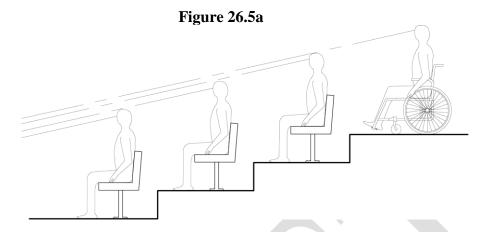
b. Where spectators are provided lines of sight over the shoulders and between the heads of spectators seated in the first row in front of their seats, spectators seated in wheelchair spaces shall be afforded lines of sight over the shoulders and between the heads of seated spectators in the first row in front of wheelchair spaces. See **Figure 26.5b**.
