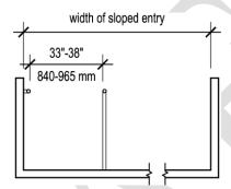
e. Handrail extensions specified by **521CMR 12.00: RAMPS** shall not be required at the bottom landing serving a sloped entry.
