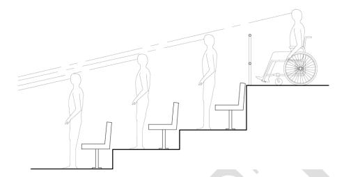
b. Where standing spectators are provided lines of sight over the shoulders and between the heads of spectators standing in the first row in front of their seats, spectators seated in wheelchair spaces shall be afforded lines of sight over the shoulders and between the heads of standing spectators in the first row in front of wheelchair spaces. See **Figure 26.5d**.
