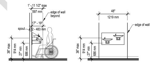
c. Where a drinking fountain is located in a recess and has no knee clearance below, the recess depth shall not exceed the fountain depth and the fountain shall have a *clear floor or ground space* that allows a person in a wheelchair to make a parallel approach to the unit (See **Figure 17.2d**). This *clear floor or ground space* shall comply with **521 CMR 6.1**, **Clear Floor or Ground Space for Wheelchairs**.
