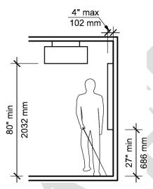
8.6.2 Objects mounted with their leading edges at or below 27 inches (686 mm) above the finished floor may protrude any distance as long as they do not reduce the *accessible route* to less than 36 inches (914 mm) *clear* width. See **Figure 8.6c**.
