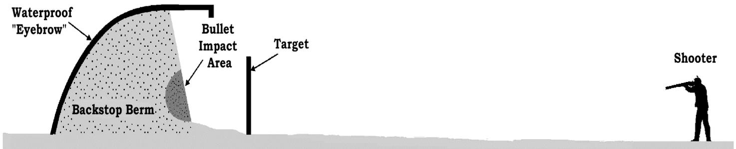
**Side view of a rifle/pistol range backstop. An "eyebrow" prevents precipitation from eroding the backstop and helps to contain ricochets. Figure adapted from *Environmental Aspects of Construction and Management of Outdoor Shooting Ranges*, National Shooting Sports Foundation, 1997.**
