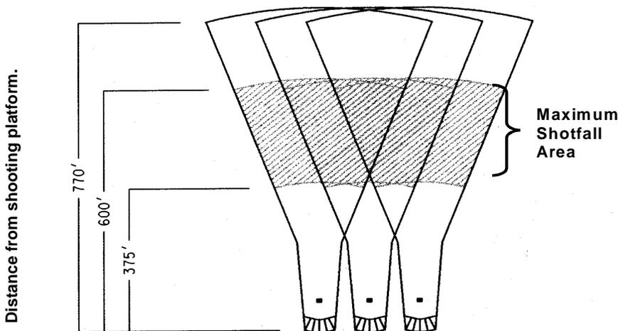
**Lead trap loads can travel 770 feet, with most shot landing between 375 and 600 feet from the shooter. The shotfall zone for a single trap field covers about 4 acres. Each additional trap field adds ~ 1 $\frac{3}{4}$  acres to the fall zone (assuming the trap houses are 100 feet apart). Figure adapted from *Environmental Aspects of Construction and Management of Outdoor Shooting Ranges*, National Shooting Sports Foundation, 1997.**
